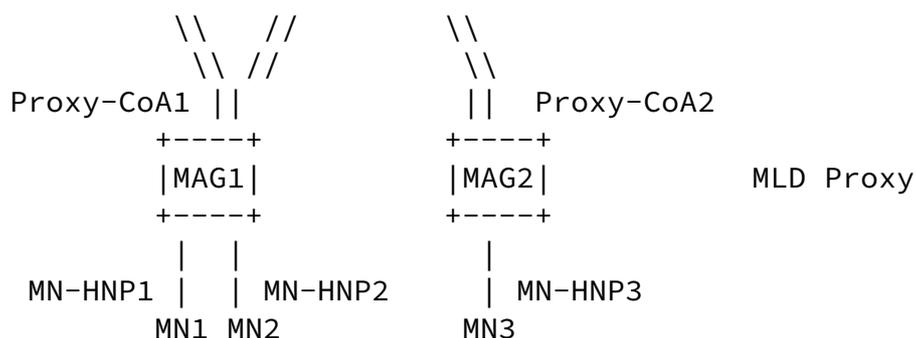
Figure 1: Reference Network for Multicast Deployment in PMIPv6
