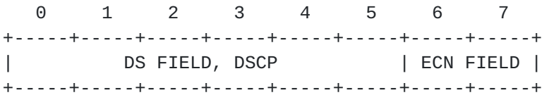
Figure 4: The Differentiated Services and ECN Fields in IP
