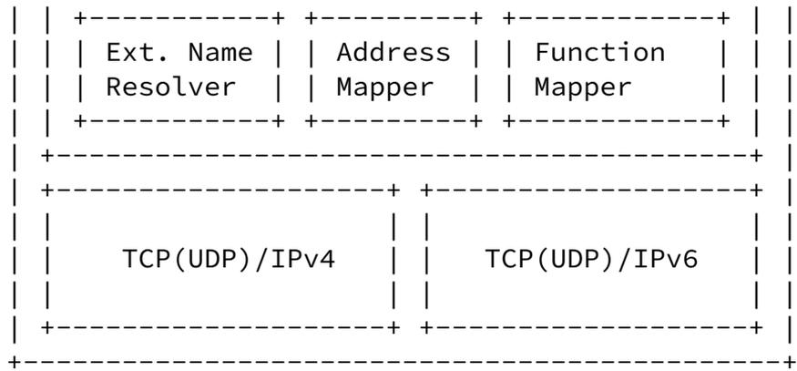
Figure 1: Architecture of a dual-stack host using protocol translation at the socket layer
