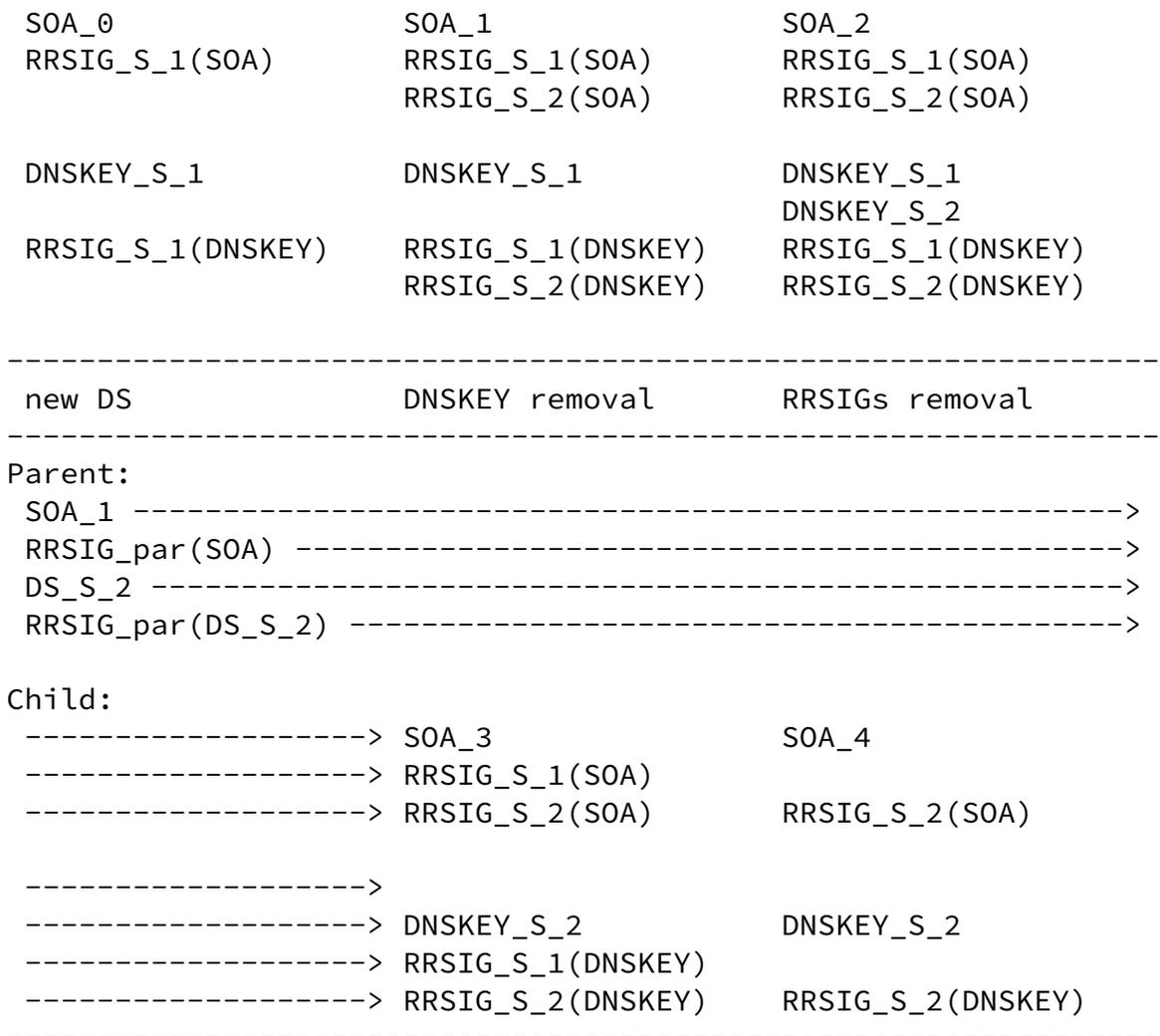
Figure 12: Single-Type Signing Scheme Algorithm Roll
