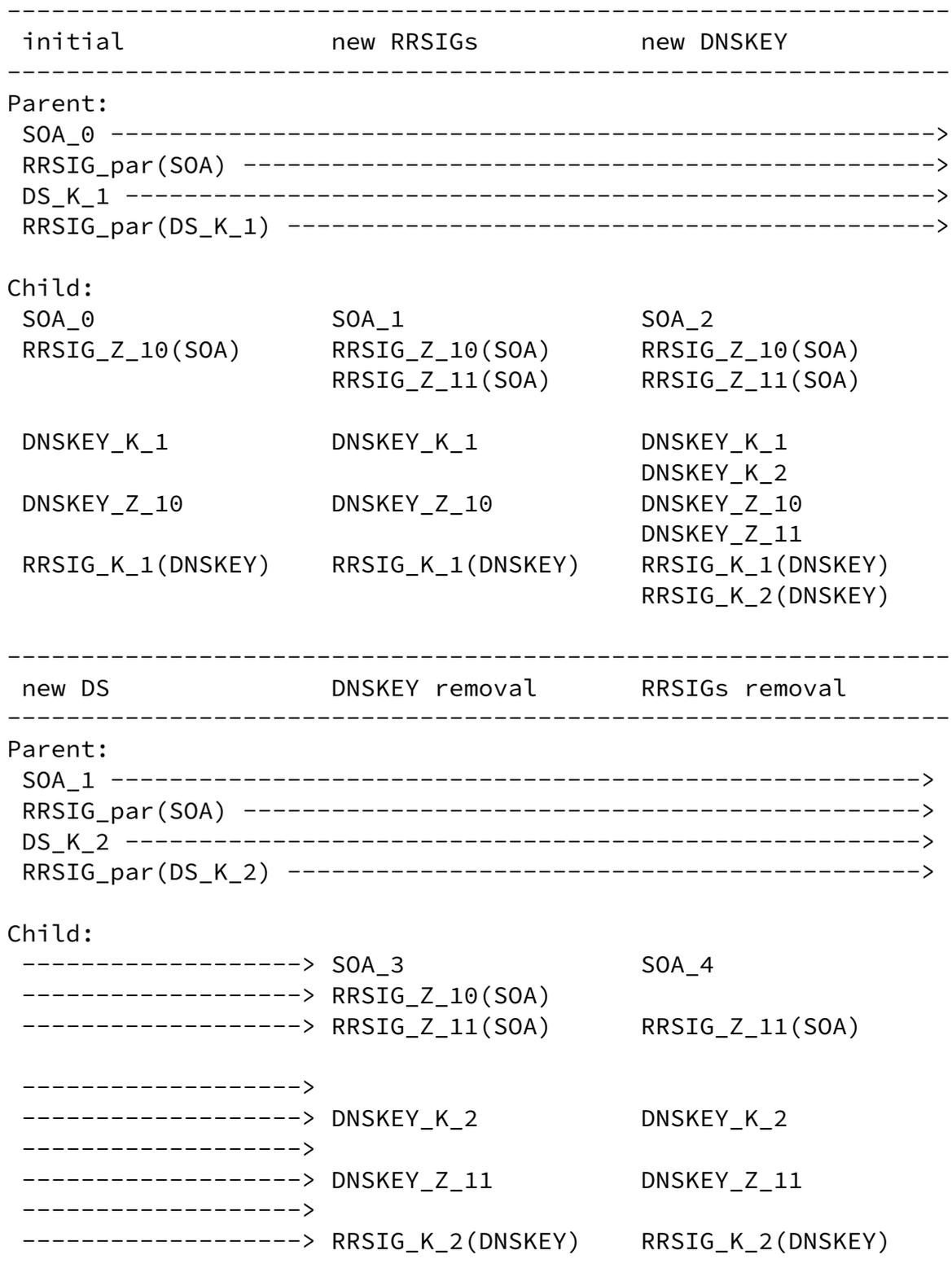
Figure 8: Stages of Deployment during an Algorithm Rollover
