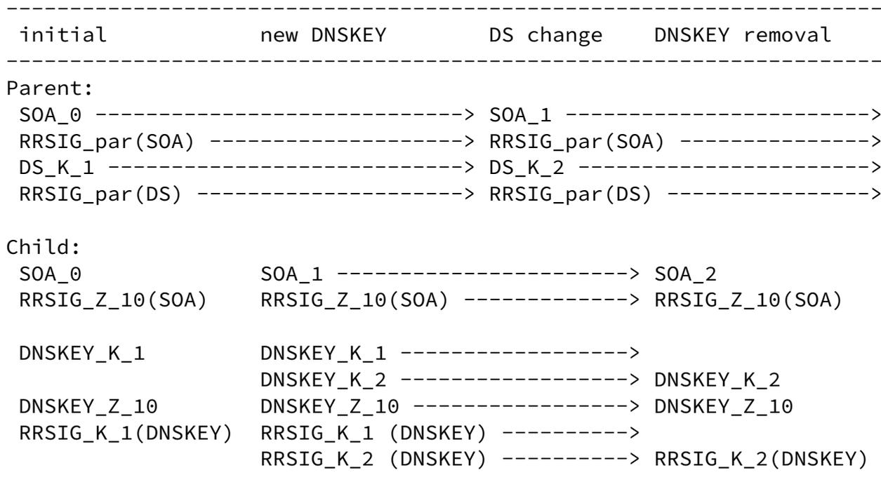
Figure 4: Stages of Deployment for a Double-Signature Key Signing Key Rollover
