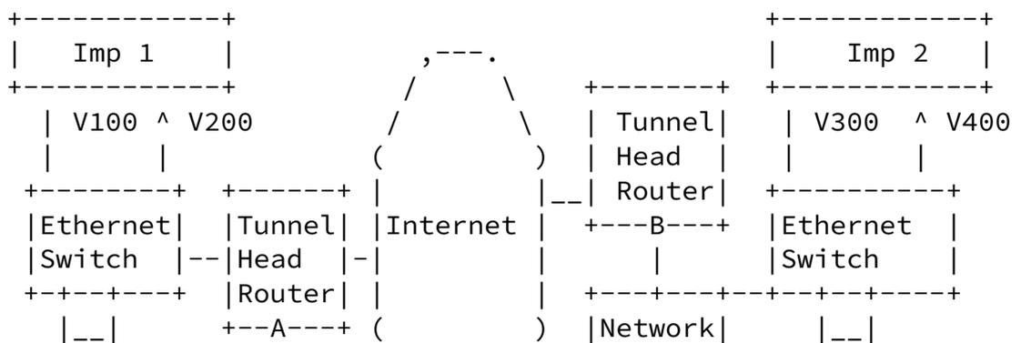
site. Thus, test streams traverse the L2TP tunnel twice but appear to be one-way tests from the point of view of the test equipment.
