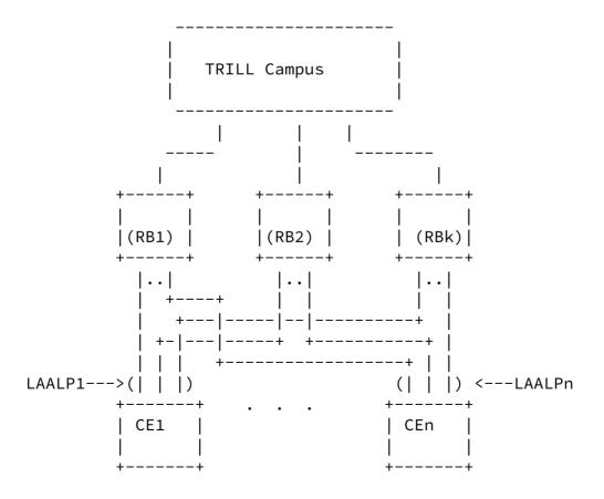
Figure 1: Active-Active Connection to TRILL Edge RBridges
