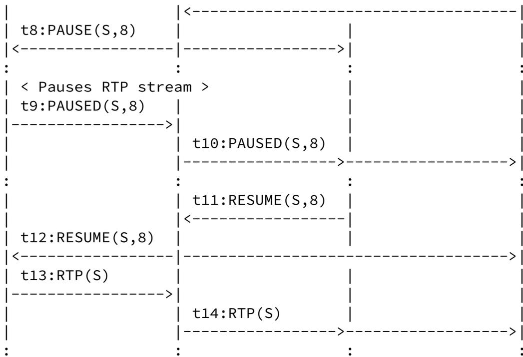
Figure 19: Pause and Resume Operation between One Sender and Two Receivers through Relay
