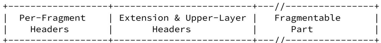
The Per-Fragment headers must consist of the IPv6 header plus any extension headers that must be processed by nodes en route to the destination, that is, all headers up to and including the Routing header if present, else the Hop-by-Hop Options header if present, else no extension headers.
