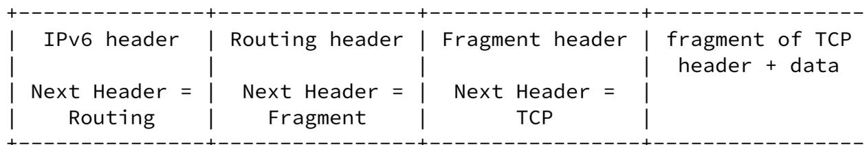
Extension headers (except for the Hop-by-Hop Options header) are not processed, inserted, or deleted by any node along a packet's delivery path, until the packet reaches the node (or each of the set of nodes, in the case of multicast) identified in the Destination Address field of the IPv6 header.
