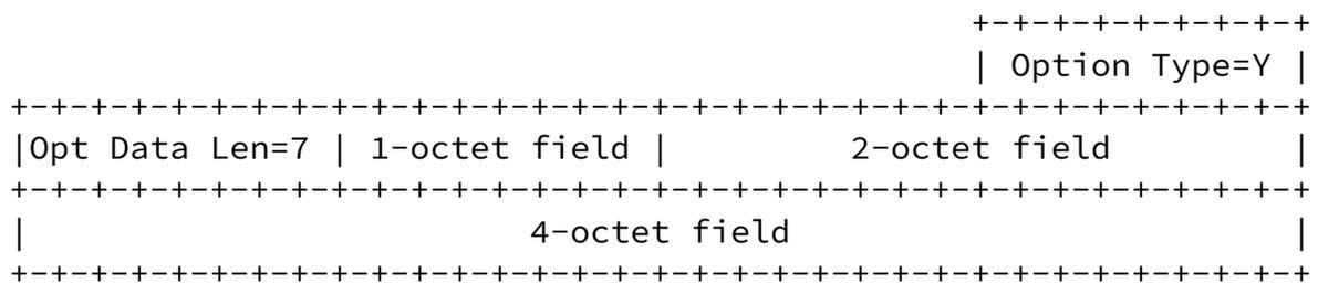
Its alignment requirement is  $4n+3$ , to ensure that the 4-octet field starts at a multiple-of-4 offset from the start of the enclosing header. A complete Hop-by-Hop or Destination Options header containing this one option would look as follows:
