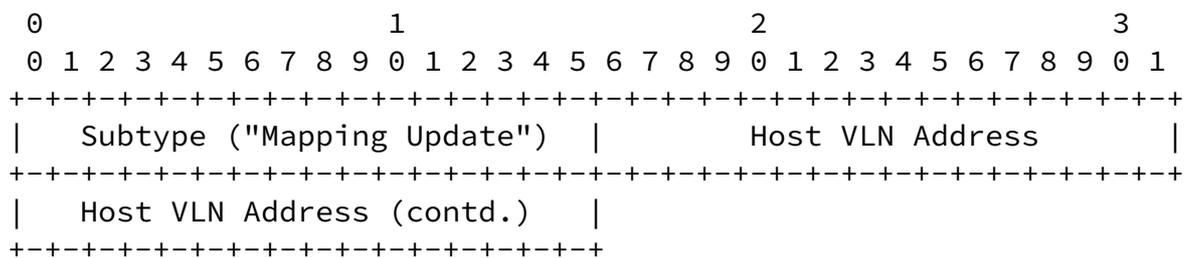
When a local VLN component receives an Ethernet frame with type
