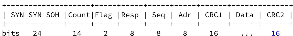
With respect to this diagram, each octet is transmitted starting from the leftmost octet, with the bits of each octet transmitted low-order bit first. The contents of all fields except the "Data" field are managed by the interface. The Internet datagram is placed in this field as-is, with no character or bit stuffing (the extent of this field is indicated by the interface in the "Count" field).
