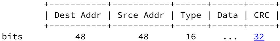
With respect to this diagram, each field is transmitted starting from the leftmost field, with the bits of each field transmitted low-order bit first. The "Dest Addr" and "Srce Addr" contain 48-bit Ethernet addresses, while the "Type" field contains the assigned value for IP datagrams (0800 hex) or for
