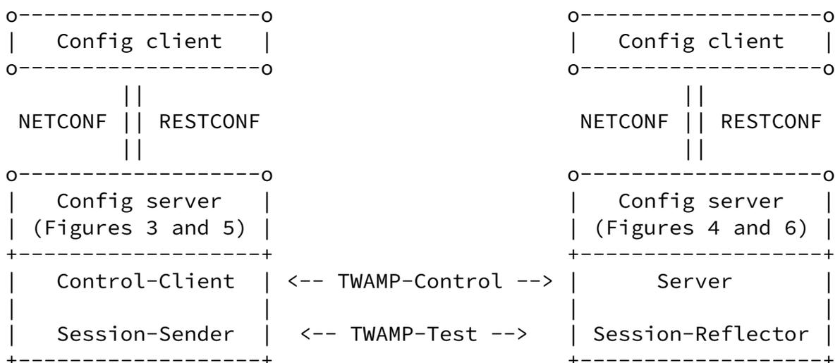
Figure 2: Simplified TWAMP Model and Protocols
