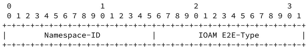
The IOAM Edge-to-Edge Option-Type IOAM-Data-Fields MUST be aligned by 4 octets:
