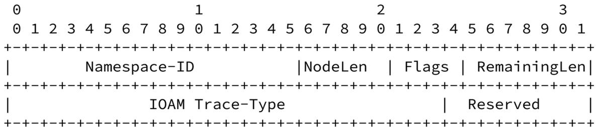
The trace option data MUST be aligned by 4 octets:
