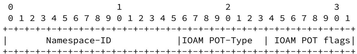
IOAM Proof of Transit Option-Type IOAM-Data-Fields MUST be aligned by 4 octets:
