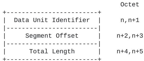
Figure 7-4. PDU Header--Segmentation Part
