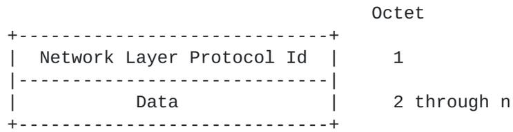
Figure 7-9. Inactive Network Layer Protocol
