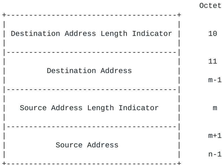
Figure 7-3. PDU header--Address Part
