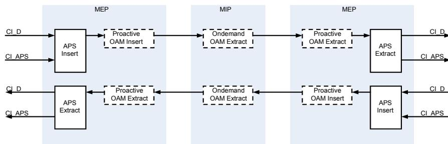
Figure 8-16/ – Overview of the processes involved with APS function
