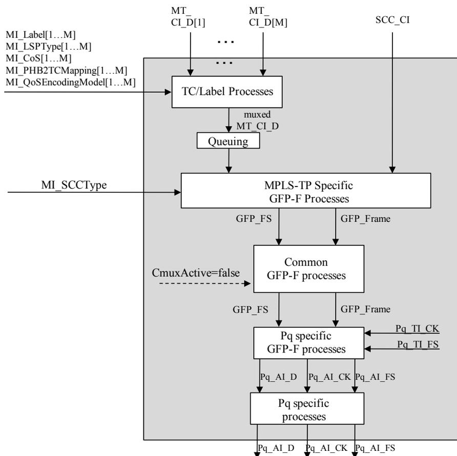
Figure 11-30/G.8121/Y.1381 – Pq/MT\_A\_So process diagram
