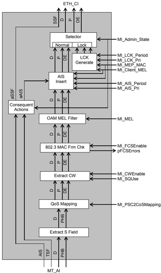
Figure 10-4/G.8121/Y.1381 – MT/ETH\_A\_Sk process diagram
