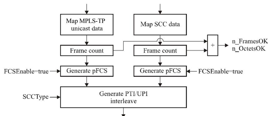
Figure 8-7/G.8121/Y.1381 – MPLS-TP-specific GFP-F source process
