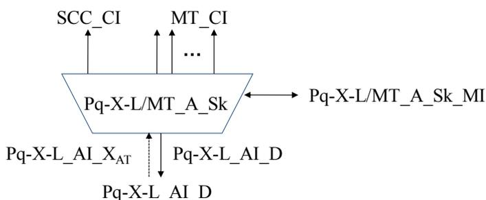
Figure 11-35/G.8121/Y.1381 – Pq-X-L/MT\_A\_Sk symbol
