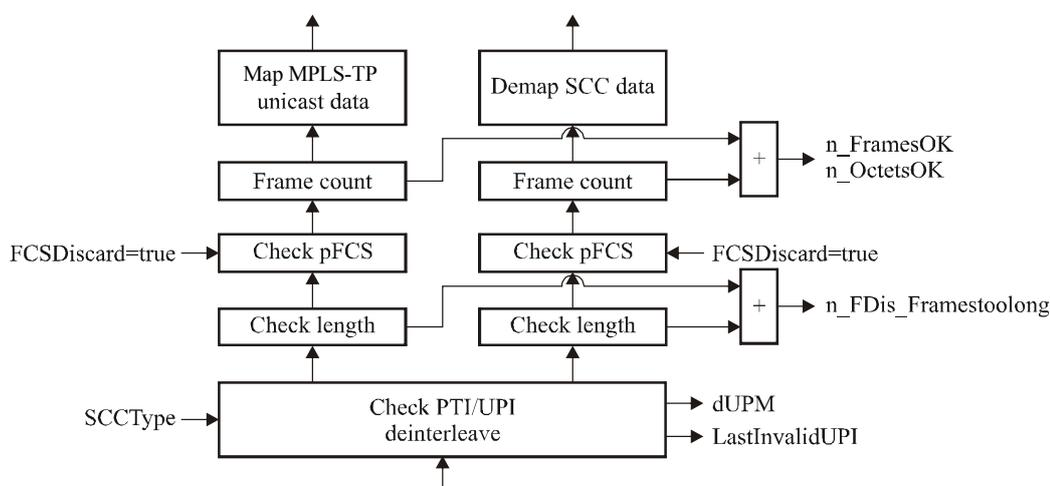
Figure8-8/G.8121/Y.1381 – MPLS-TP-specific GFP-F sink process
