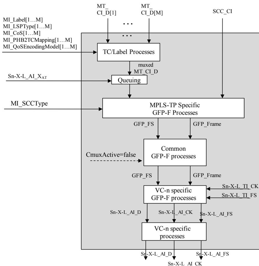
**Figure 11-2/G.8121/Y.1381 – Sn/MT\_A\_So process diagram**
