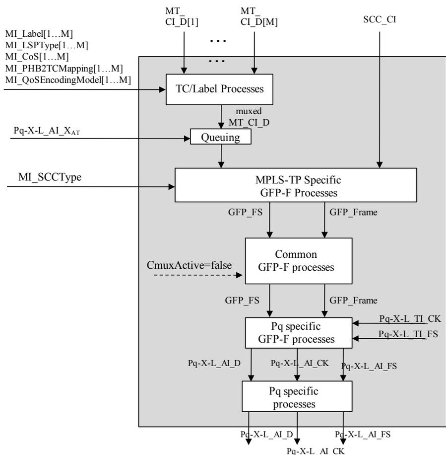
Figure 11-34/G.8121/Y.1381 – Pq-X-L/MT\_A\_So process diagram
