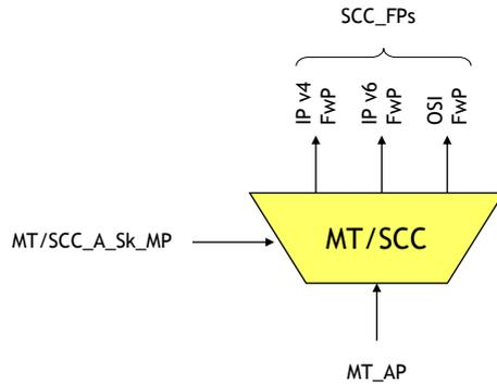
**Figure 10-8/G.8121/Y.1382 – MT/SCC\_A\_Sk function**
