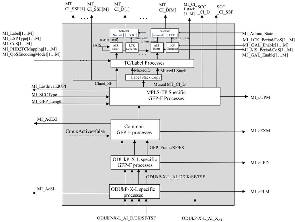
**Figure 11-27/G.8121/Y.1381 – ODUkP-X-L/MT\_A\_Sk process diagram**
