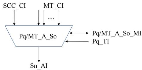
**Figure 11-29/G.8121/Y.1381 – P<sub>q</sub>/MT\_A\_So symbol**
