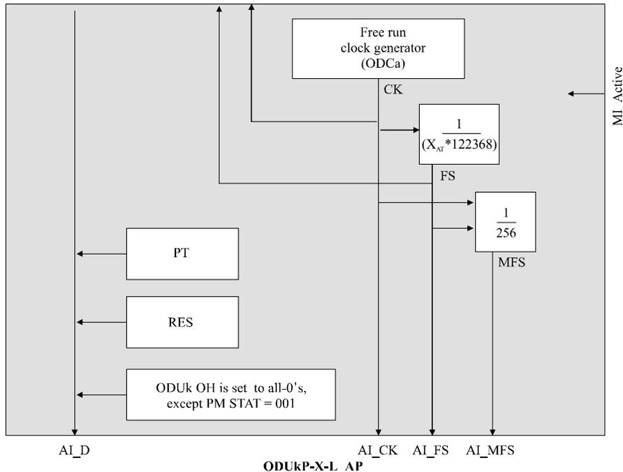
**Figure 11-25/G.8121/Y.1381 – ODUkP-X-L specific source processes**
