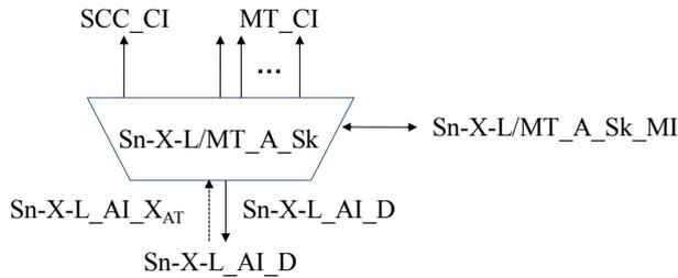
Figure 11-7/G.8121/Y.1381 – Sn-X-L/MT\_A\_Sk symbol
