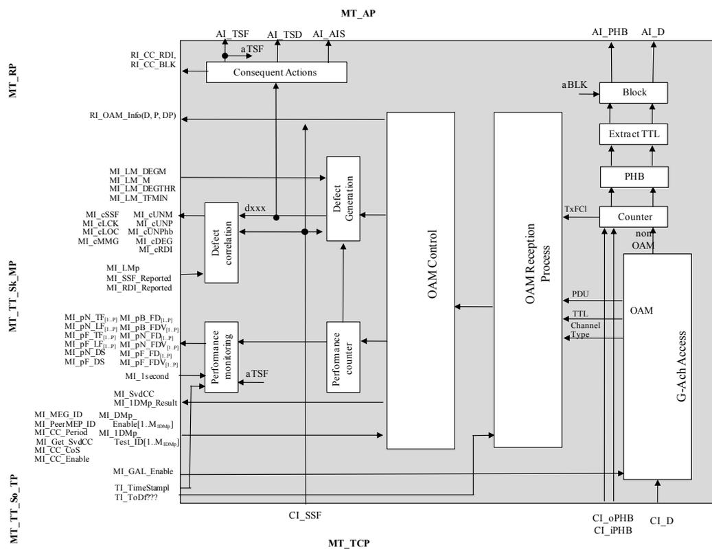
Figure 9-7/G.8121/Y.1381 – MT\_TT\_Sk process diagram
