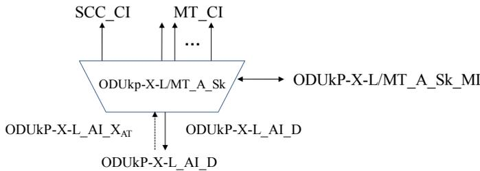
**Figure 11-26/G.8121/Y.1381 – ODUkP-X-L/MT\_A\_Sk symbol**
