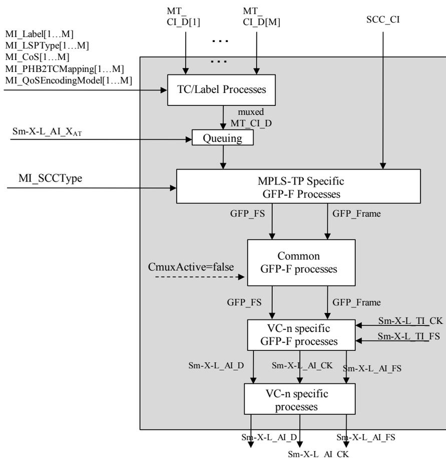
Figure 11-14/G.8121/Y.1381 – Sm-X-L/MT\_A\_So process diagram
