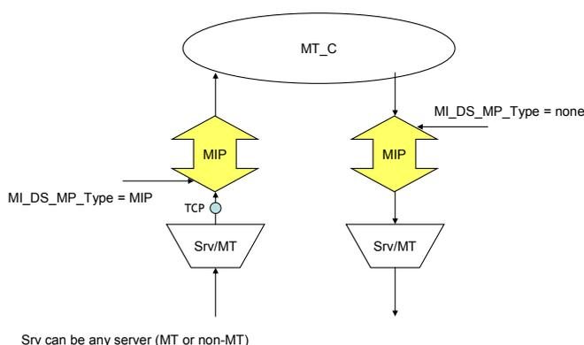
**Figure I.2 – Intermediate node with per-interface MIPs**
