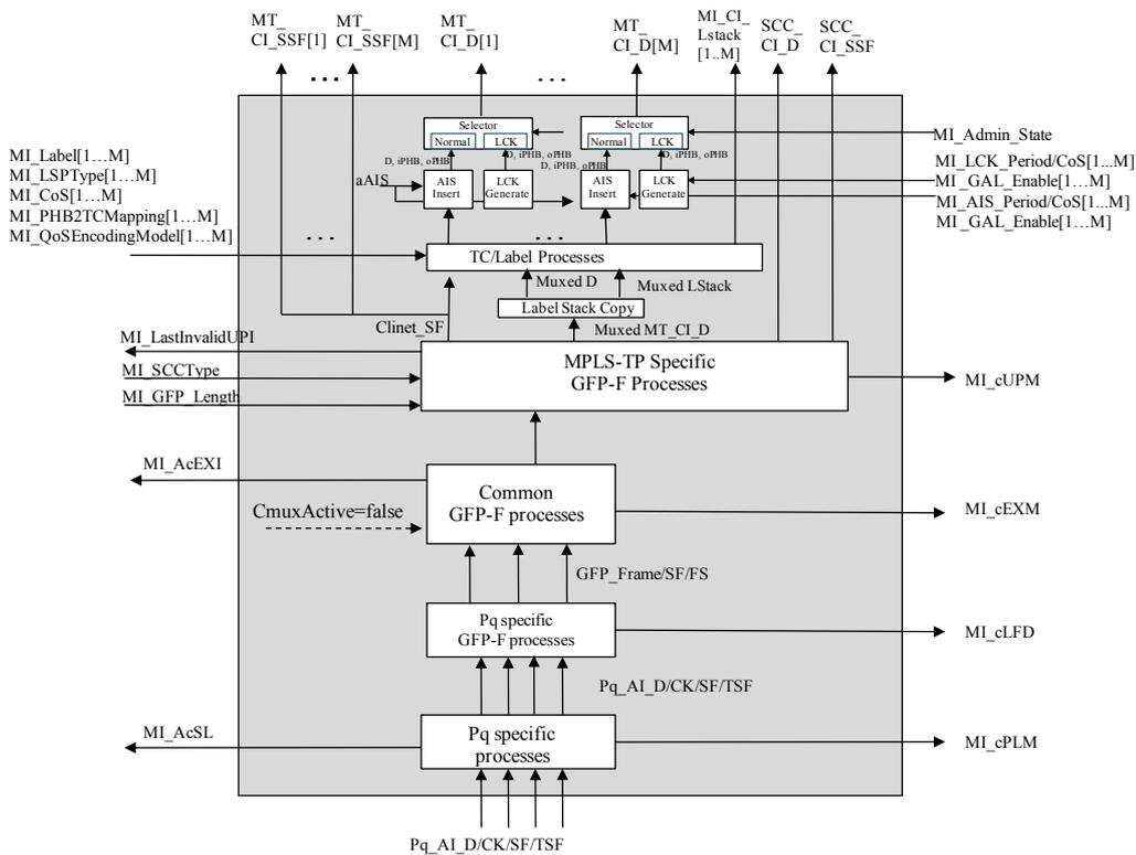
**Figure 11-32/G.8121/Y.1381 – Pq/MT\_A\_Sk process diagram**
