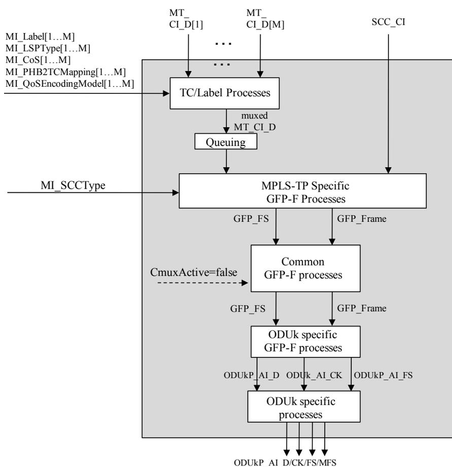
**Figure 11-18/G.8121/Y.1381 – ODUkP/MT\_A\_So process diagram**
