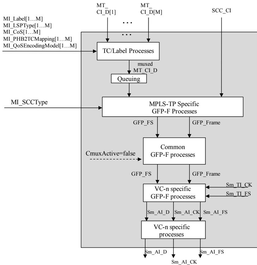
Figure 11-6/G.8121/Y.1381 – Sn-X-L/MT\_A\_So process diagram
