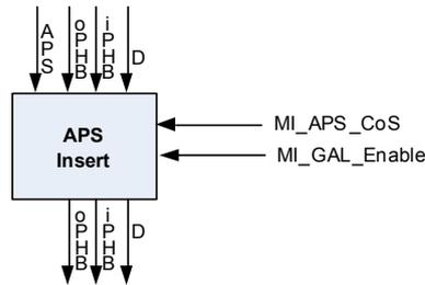
**Figure 8-17/G.8121/Y.1381 – APS Insert process**
