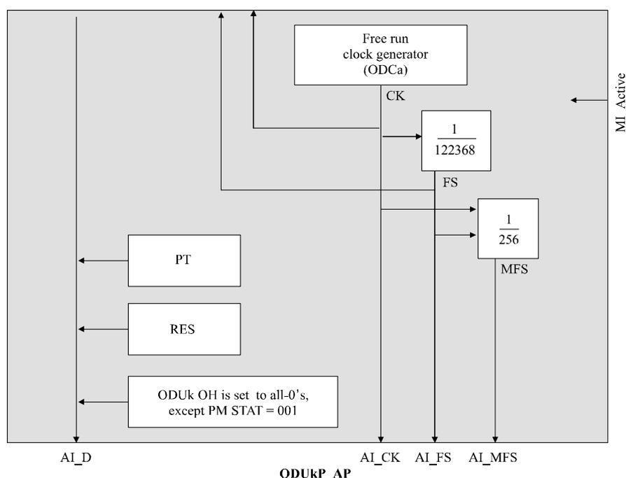
**Figure 11-19/G.8121/Y.1381 – ODUkP specific source processes**
