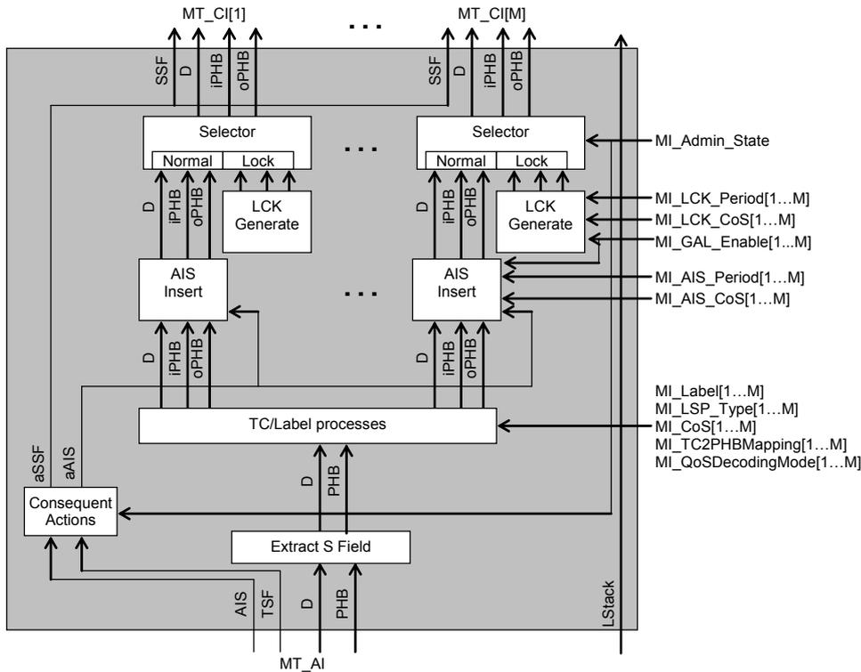
**Figure 9-11/G.8121/Y.1381 – MT/MT\_A\_Sk process diagram**
