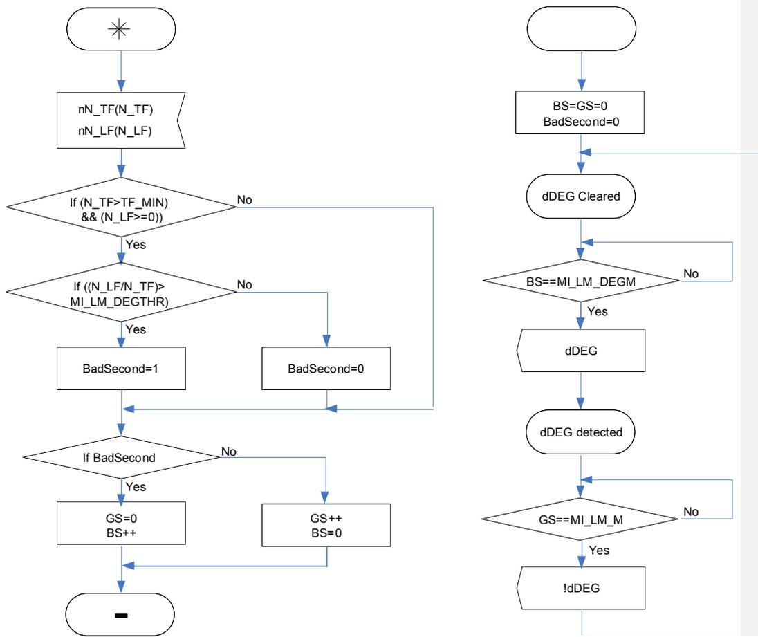
Figure 6-3/G.8121 – dDEG detection and clearance process
