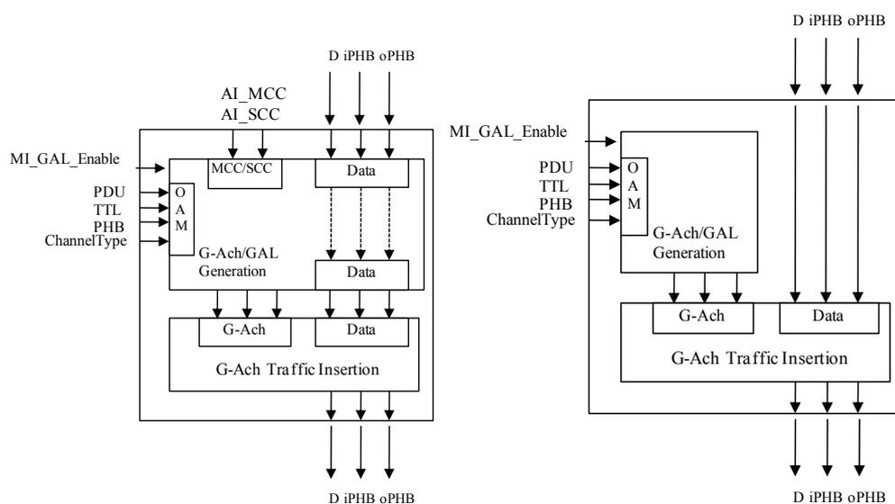
**Figure 8-1 – G-ACh Insertion Process**
