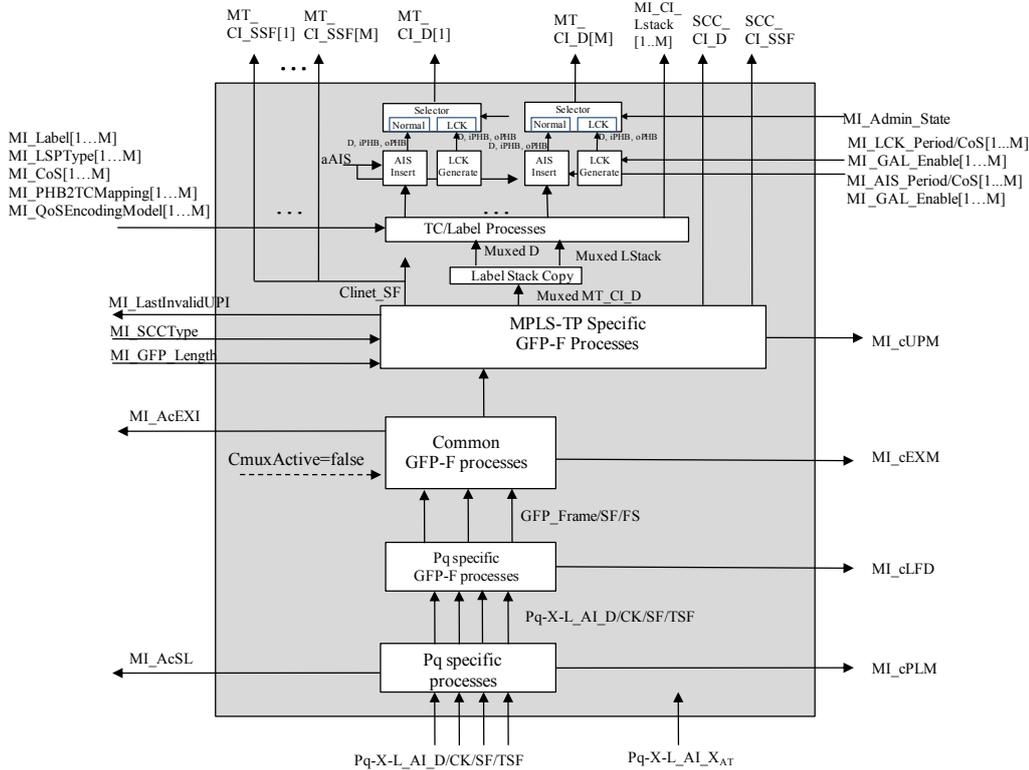
**Figure 11-36/G.8121/Y.1381 – Pq-X-L/MT\_A\_Sk process diagram**
