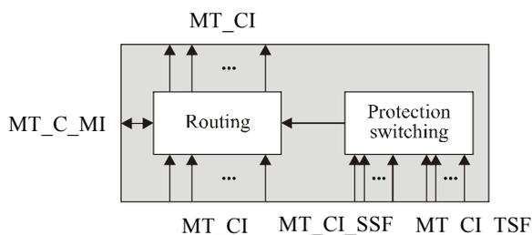
**Figure 9-2/G.8121/Y.1381 – MT\_C process diagram**
