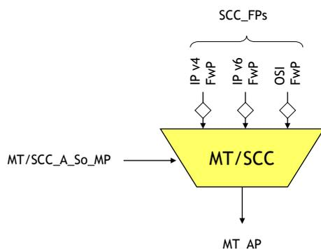
**Figure 10-6/G.8121/Y.1382 – MT/SCC\_A\_So function**
