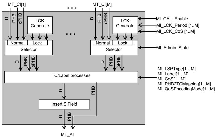
Figure 9-9/G.8121/Y.1381 – MT/MT\_A\_So process diagram
