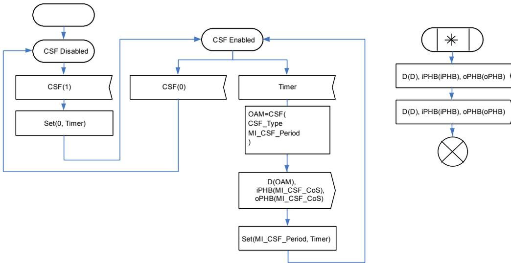
**Figure 8-23/G.8121/Y.1381 – CSF Insert behaviour**
