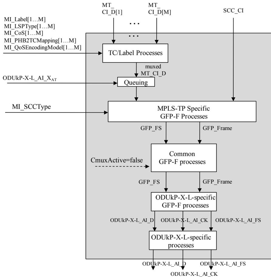
**Figure 11-24/G.8121/Y.1381 – ODUkP-X-L/MT\_A\_So process diagram**
