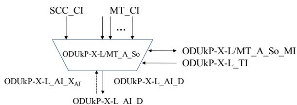
**Figure 11-23/G.8121/Y.1381 – ODUkP-X-L/MT\_A\_So symbol**
