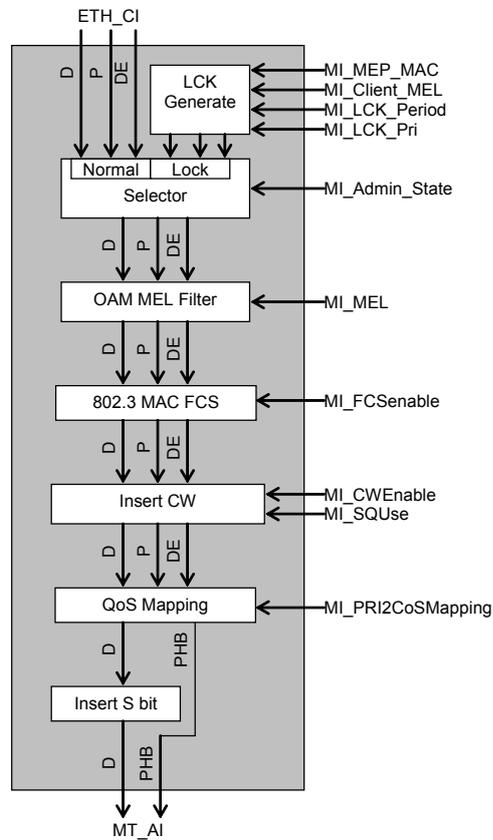
**Figure 10-2/G.8121/Y.1381 – MT/ETH\_A\_So process diagram**
