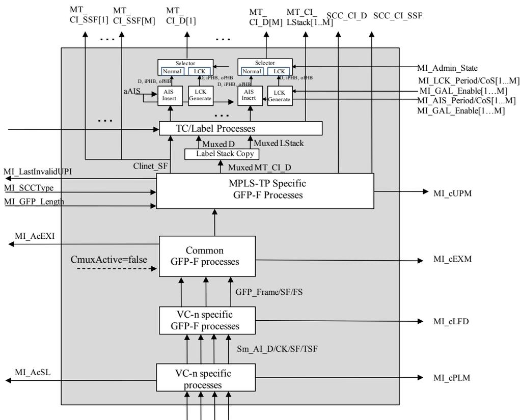
Figure 11-12/G.8121/Y.1381 – Sm/MT\_A\_Sk process diagram
