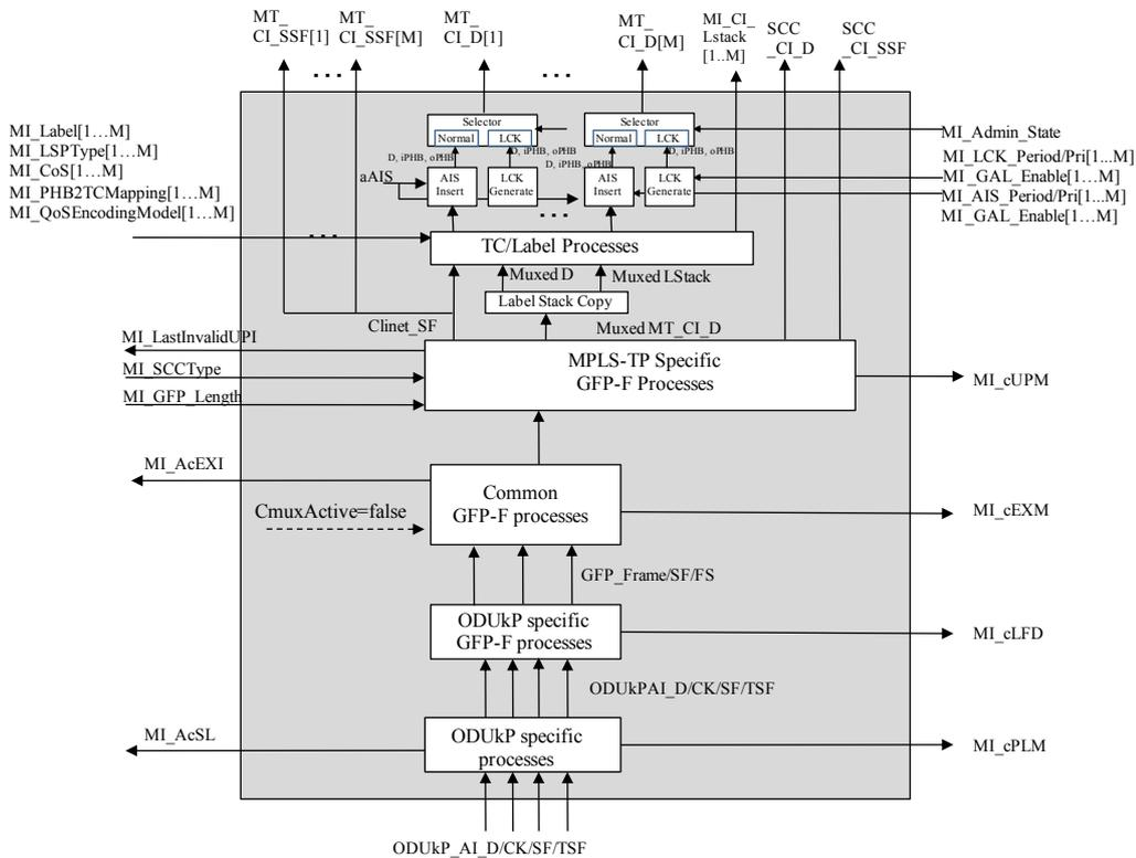
**Figure 11-21/G.8121/Y.1381 – ODUkP/MT\_A\_Sk process diagram**
