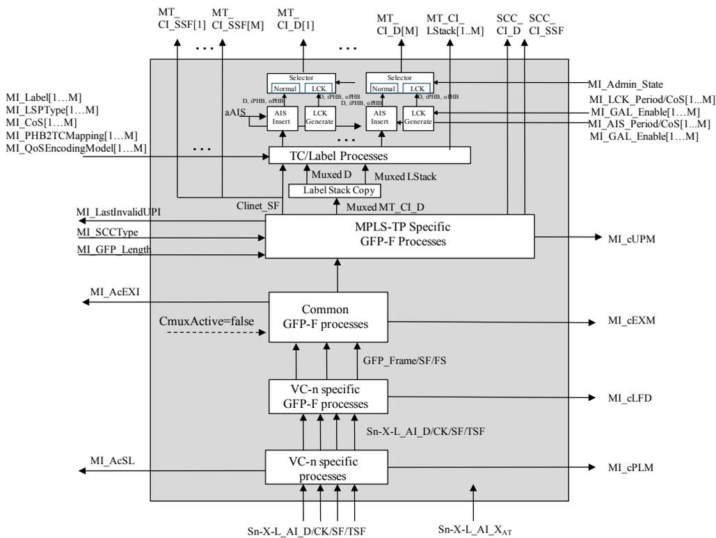
Figure 11-8/G.8121/Y.1381 – Sn-X-L/MT\_A\_Sk process diagram
