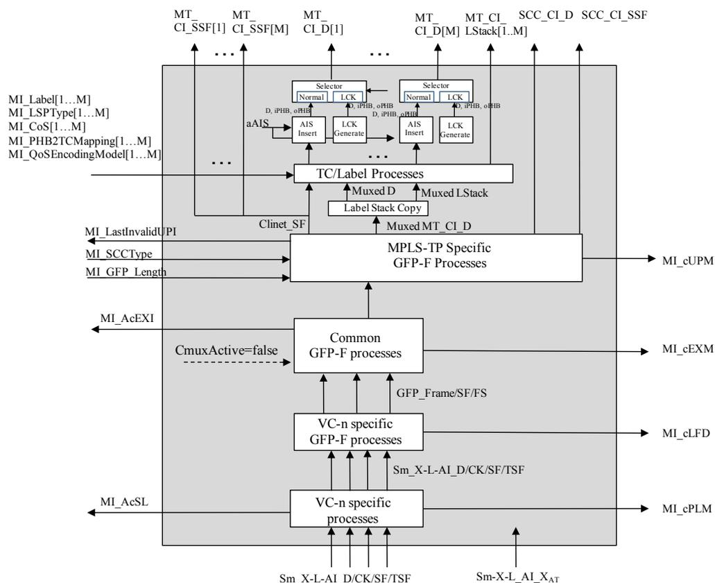
**Figure 11-16/G.8121/Y.1381 – Sm-X-L/MT\_A\_Sk process diagram**
