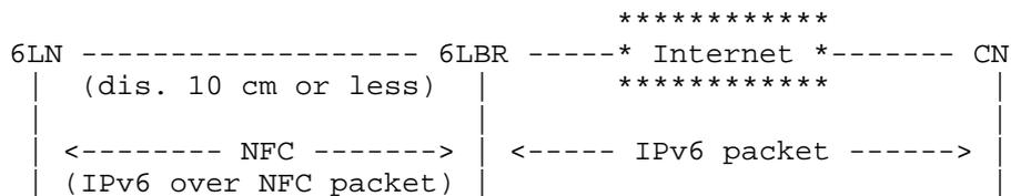
Figure 10: NFC-enabled device network connected to the Internet
