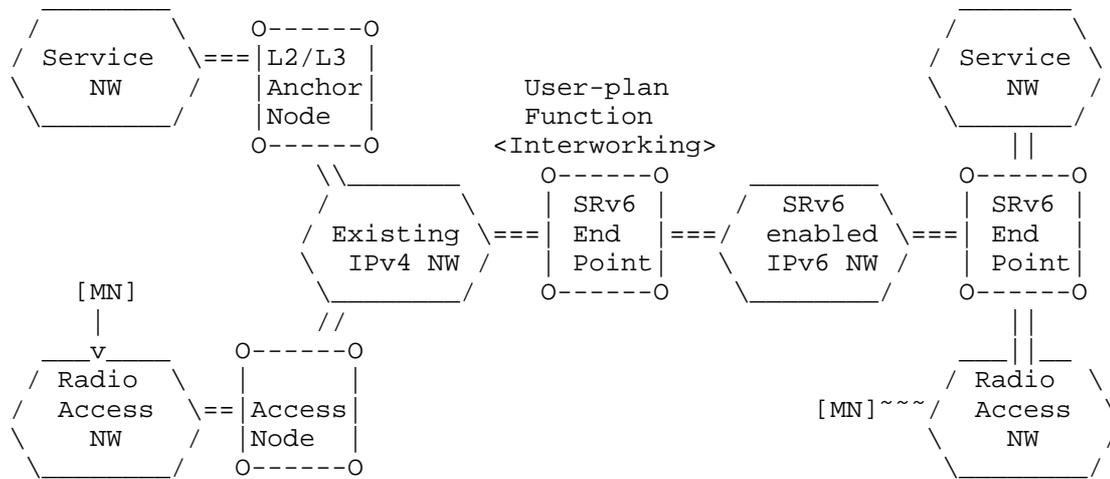
Figure 2: Interworking with Existing Mobile Networks
