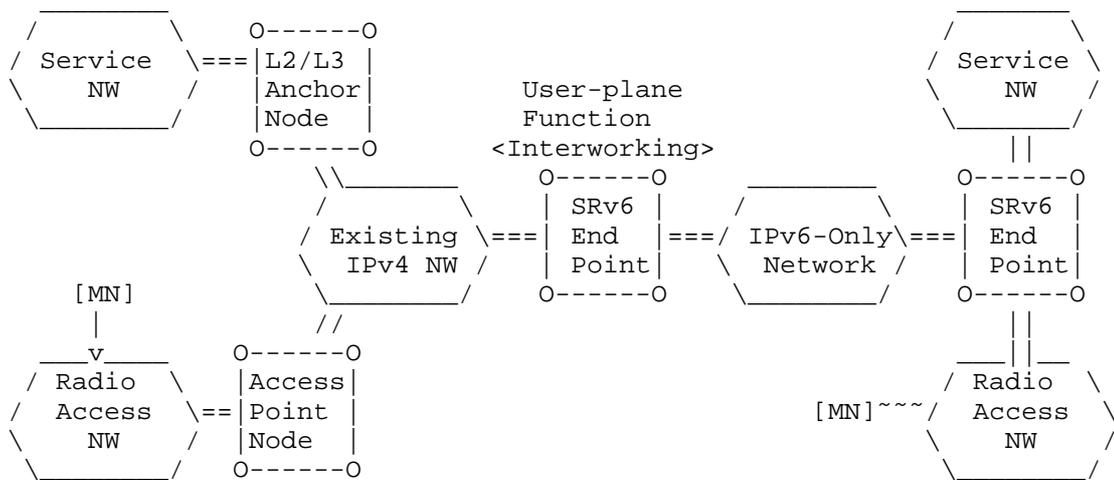
Figure 2: Interworking with Existing Mobile Networks
