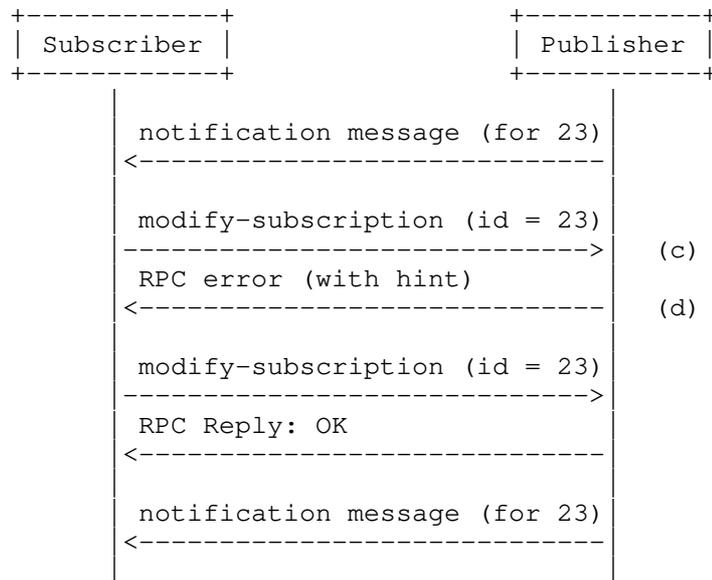
Figure 6: Interaction model for successful subscription modification
