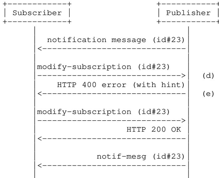
Figure 7: Interaction model for successful subscription modification
