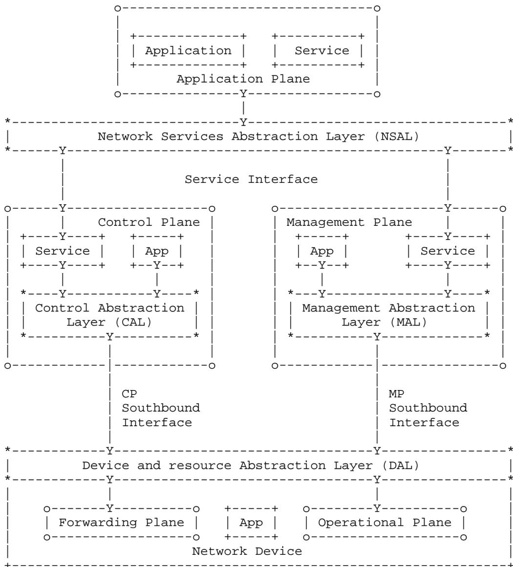
Figure 4: SDN Layer Architecture
