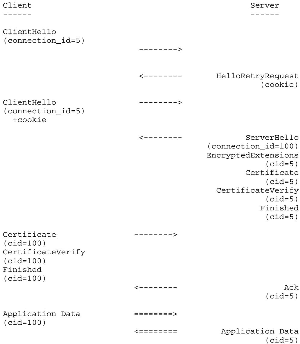
Figure 3: Example DTLS 1.3 Exchange with Connection IDs
