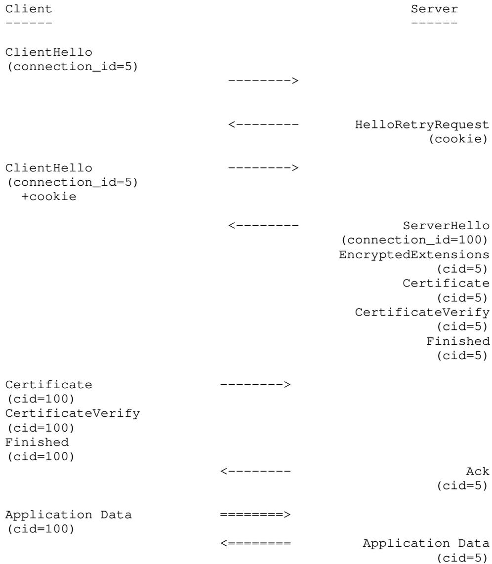
Figure 13: Example DTLS 1.3 Exchange with CIDs
