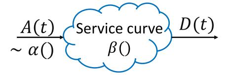
Flow is constrained by arrival curve  $\alpha()$ ; served in network element with service curve  $\beta()$ . Then
