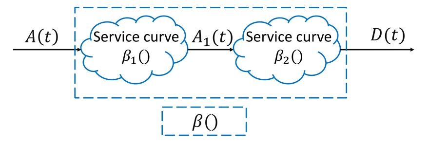
A flow is served in series, network element i offers service curve  $\beta_i()$ . The concatenation offers the service curve  $\beta()$  defined by
