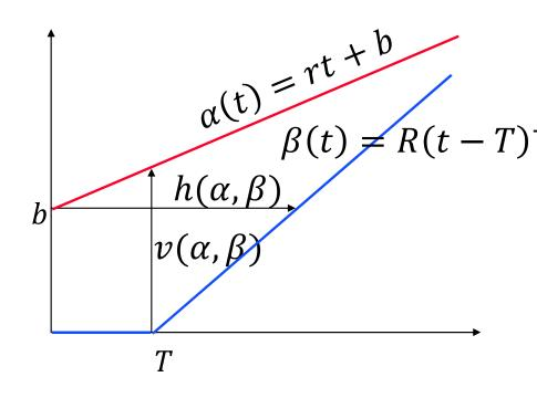
One flow, constrained by one token bucket is served in a network element that offers a rate latency service curve.
