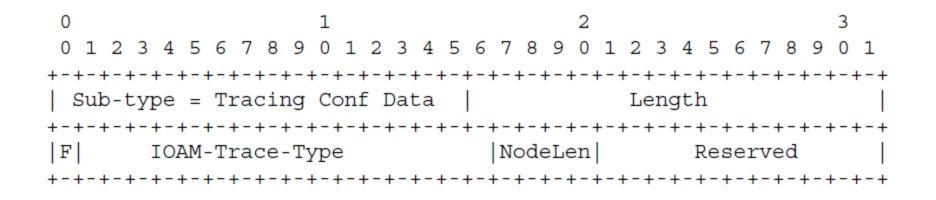
Figure 2: IOAM Tracing Configuration Data Sub-TLV
