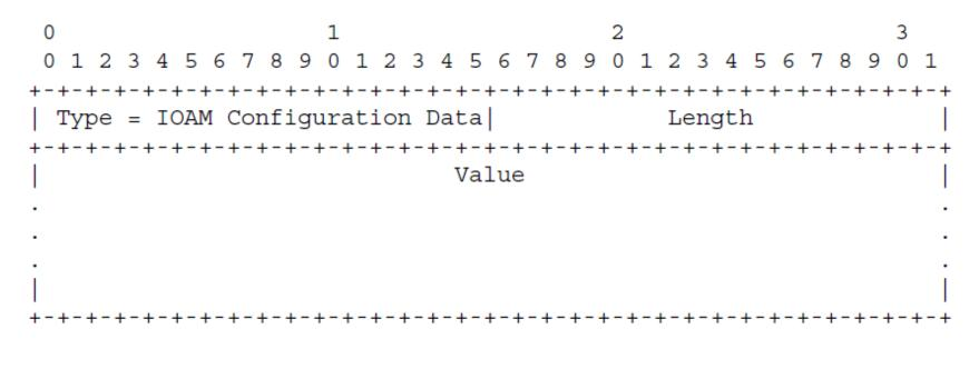
Figure 1: IOAM Configuration Data TLV
