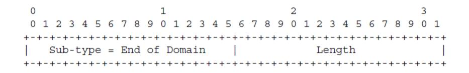
Figure 5: IOAM End of Domain Sub-TLV
