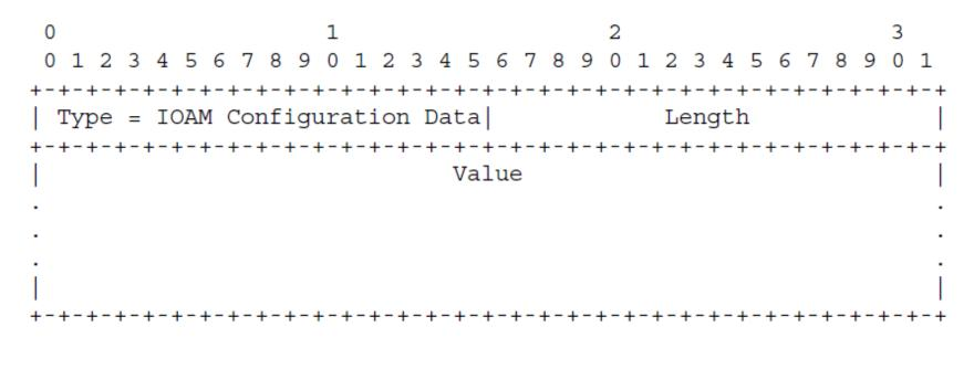
Figure 1: IOAM Configuration Data TLV
