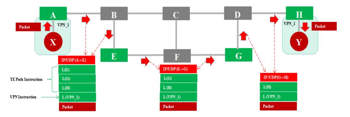
• Unified SR can be seamlessly integrated with the existing MPLS-VPN technologies by using consistent programming instructions (i.e., MPLS label stack).
