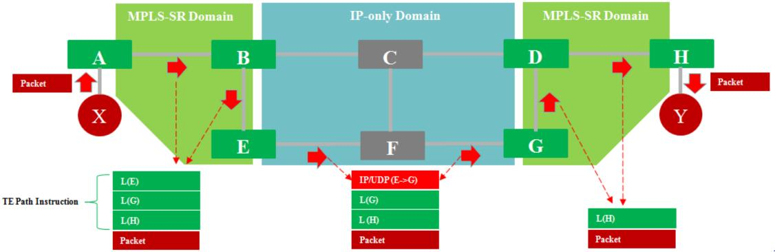
• Unified SR can be seamlessly interworking with the existing MPLS-SR technologies which greatly facilitates the incremental deployment of MPLS-SR (e.g., in the Egress Peer Engineering (EPE) case).
