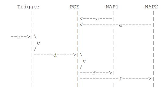
Message Sequence Chart Resulting in Pre-Warming of Routing Entries. a) subscribe to pre-warming information, b)initiate service chaining based on external mgmt. trigger, c) compute SFP, d) send SFP, e) map SFP information onto paths from incoming to ongoing NAPs, f) push path information with forwarding/path identifier and URL.
