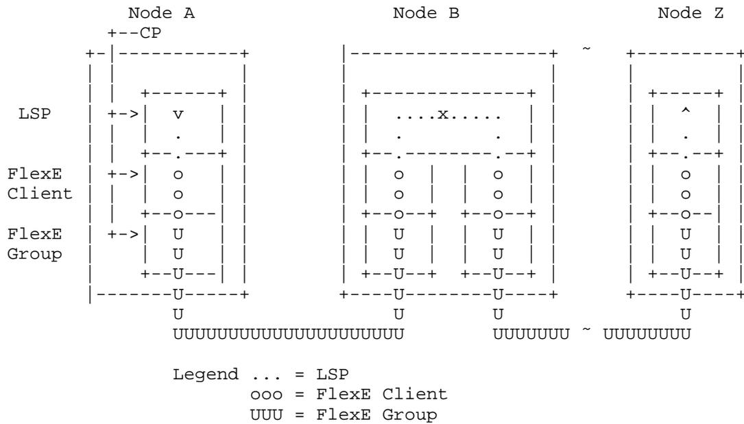
Figure 3: GMPLS controlled network with FlexE infrastructure
