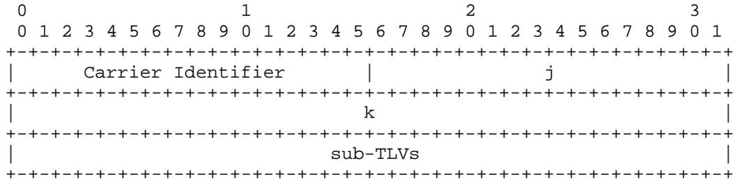
Figure 4: Sub-Carrier parameters
