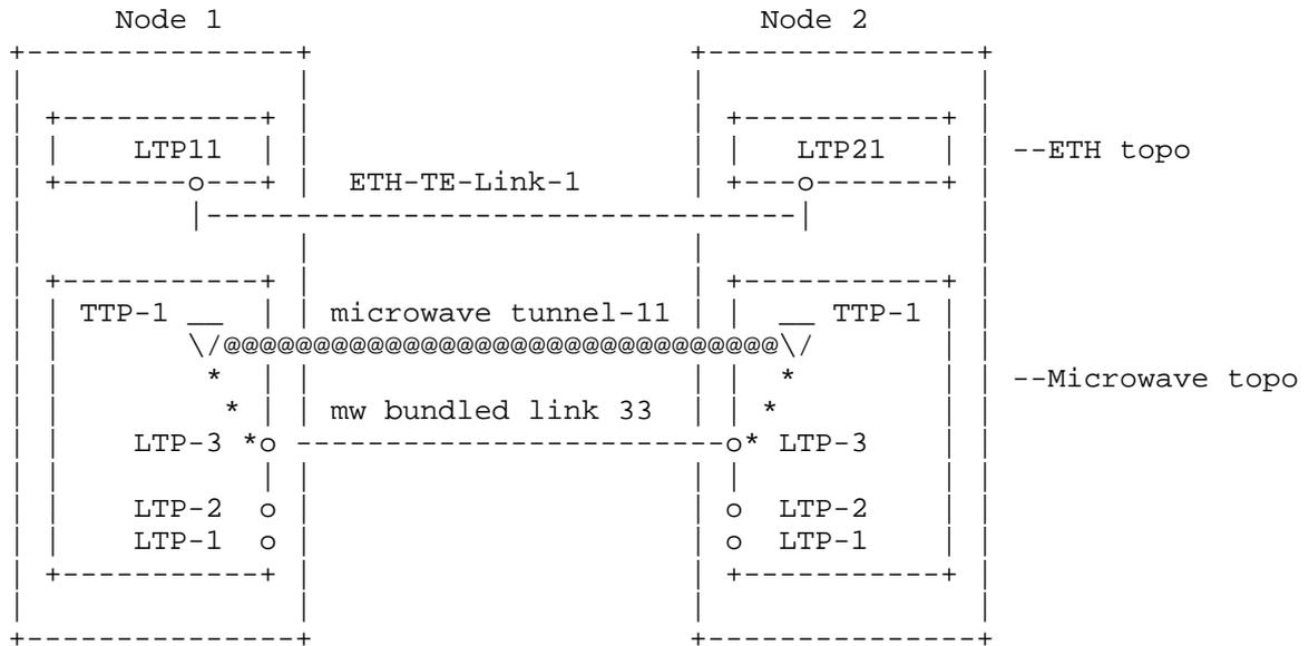
Figure 4: ETH transported on single microwave radio links
