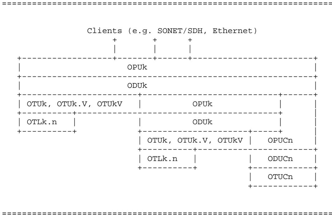
Figure 3: Digital Structure of OTN interfaces (from G.709:Figure 6-1)
