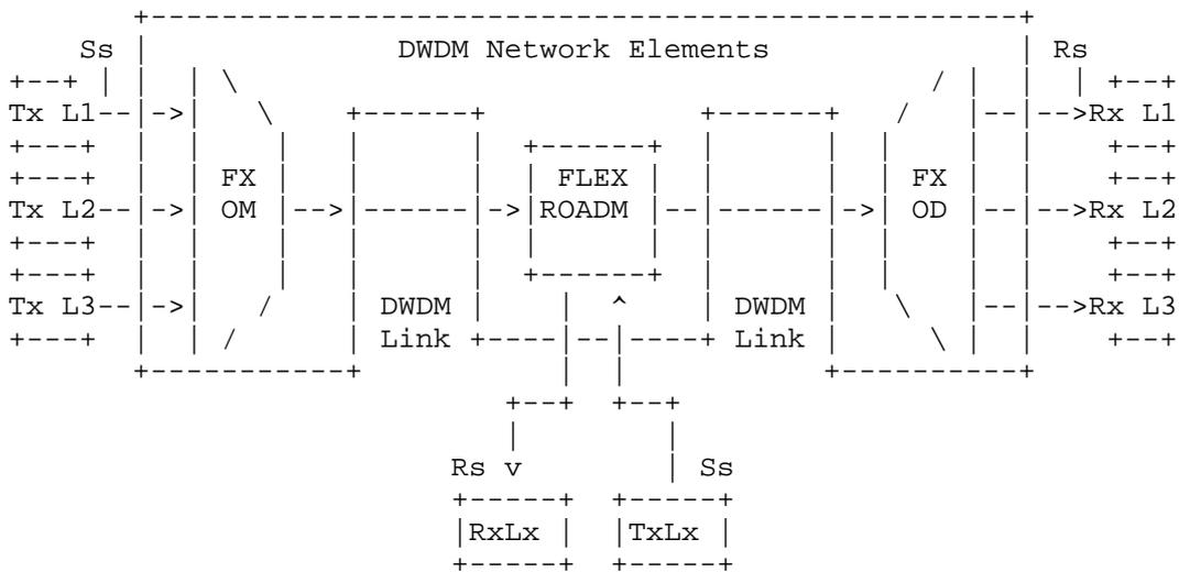
Ss = Sender reference point at the DWDM network element tributary output, this can be a set of multiple transceivers carrying the same client payload.
