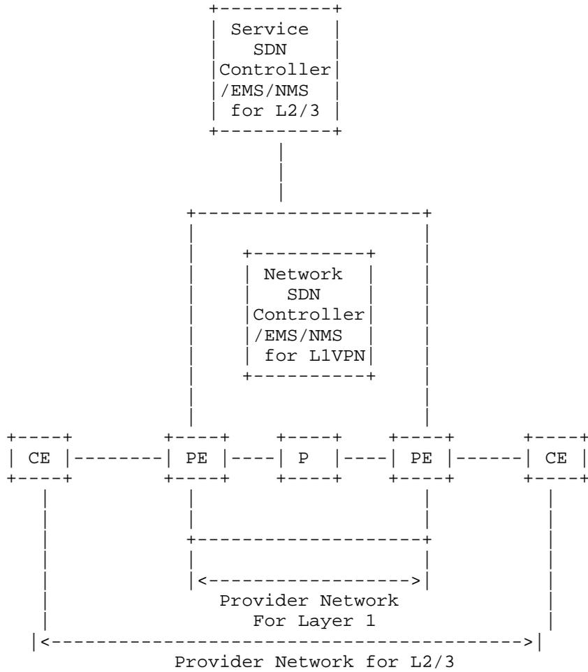
Figure 2: L1VPN SDN Controller/EMS/NMS-Based Service Model: Internal Customer
