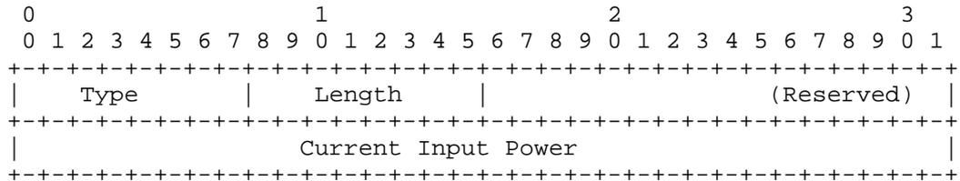
Figure 6: OCh\_Rs receive parameters
