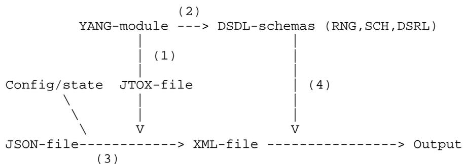
Figure 6 - DSDL-based approach for JSON code validation
