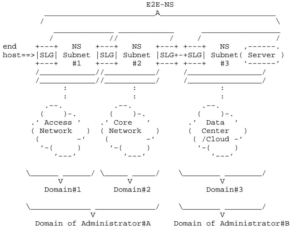
Figure 1: E2E-NS composed of multiple NS subnets
