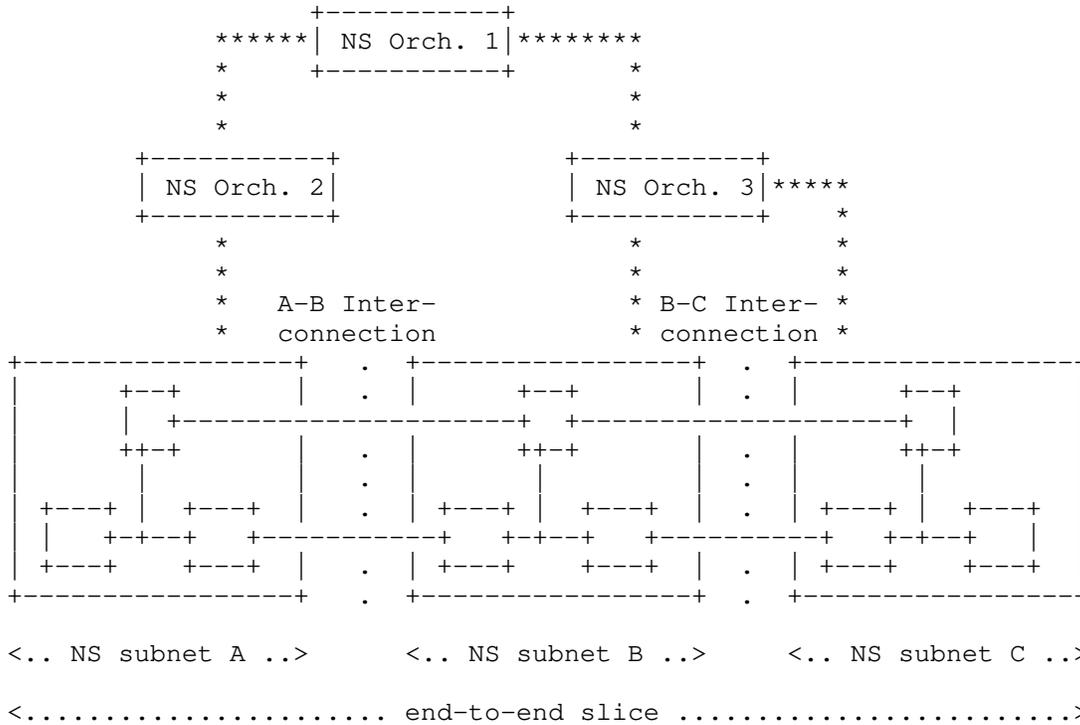
Figure 1: Overview of Network Slice Subnets Interconnection
