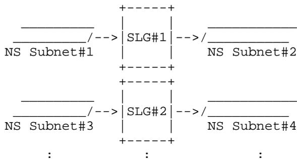
Figure 8: Overview of vertical connection of SLG: Separated Pattern
