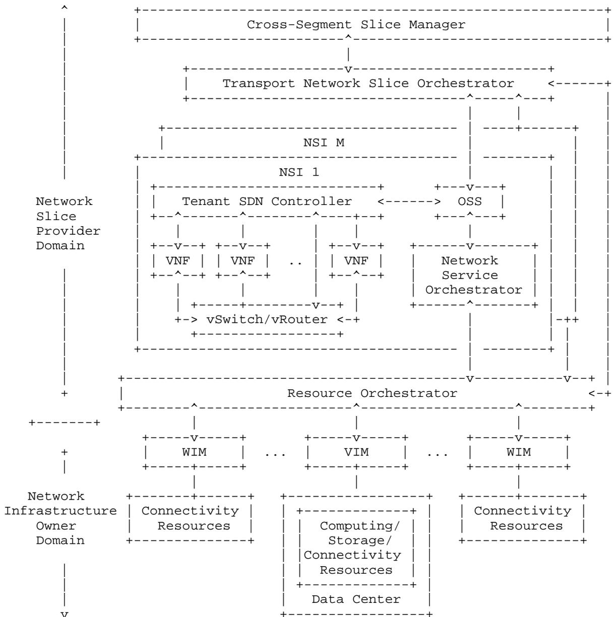
Figure 3: Integration of NFV framework in COMS architecture
