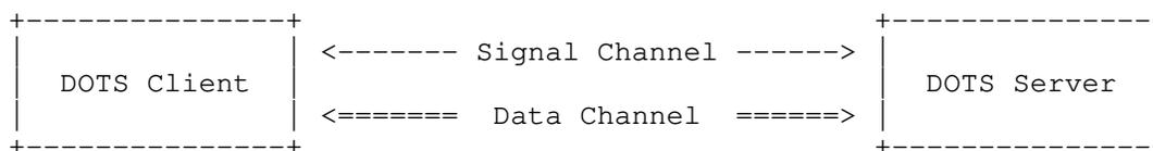
Figure 2: DOTS Interfaces
