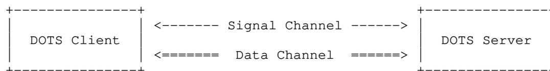
Figure 1: DOTS Channels
