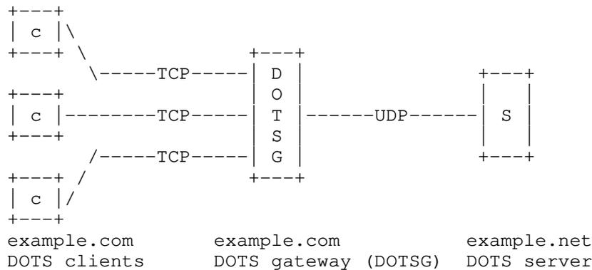
Figure 7: Client-Side Gateway with Aggregation
