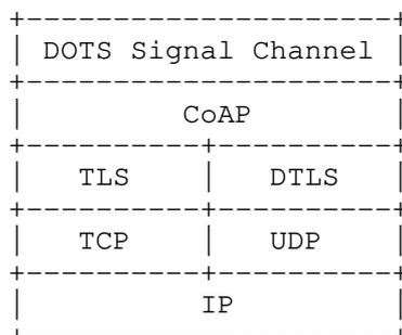
Figure 3: Abstract Layering of DOTS Signal Channel over CoAP over (D)TLS
