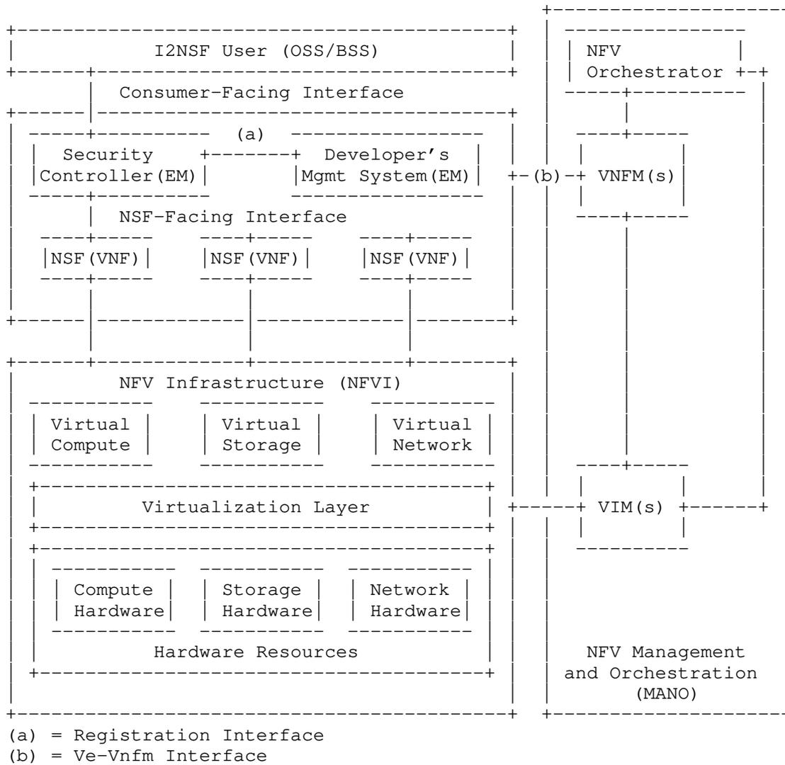
Figure 7: I2NSF Framework Implementation with respect to the NFV Reference Architectural Framework
