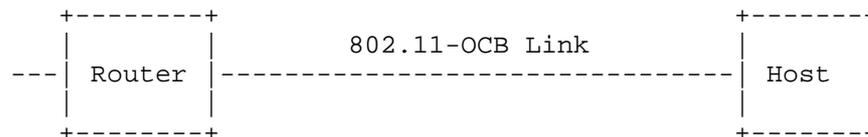
Figure 5: Topology for capturing IP packets on 802.11-OCB
