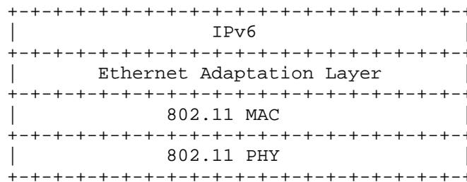
Figure 2: Ethernet Adaptation Layer stacked with other layers
