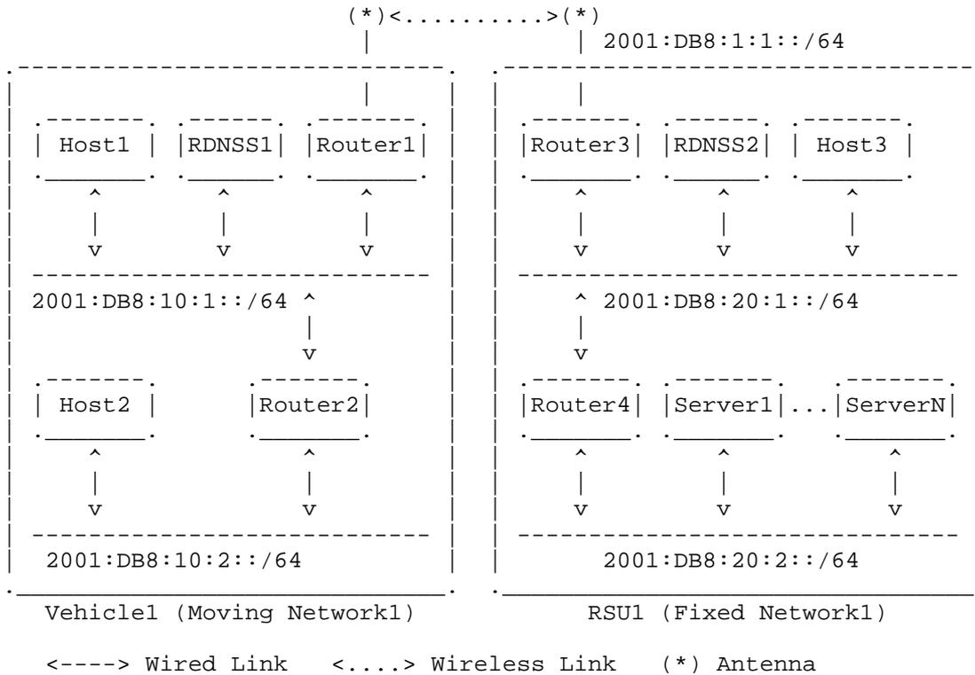
Figure 2: Internetworking between Vehicle Network and RSU Network
