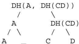
Replacing a node by \_ in TreeKEM, means performing an update on any leaf without sending the new key to the the blanked leaf. In the
