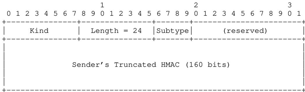
Figure 7: Join Connection (MP\_JOIN) Option (for Third ACK)
