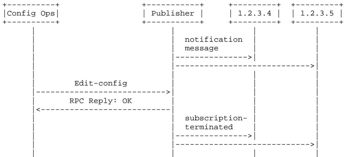
Figure 16: Interaction model for configured subscription deletion
