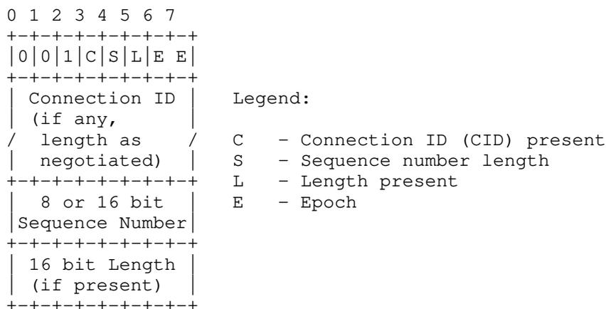
Figure 3: DTLS 1.3 CipherText Header
