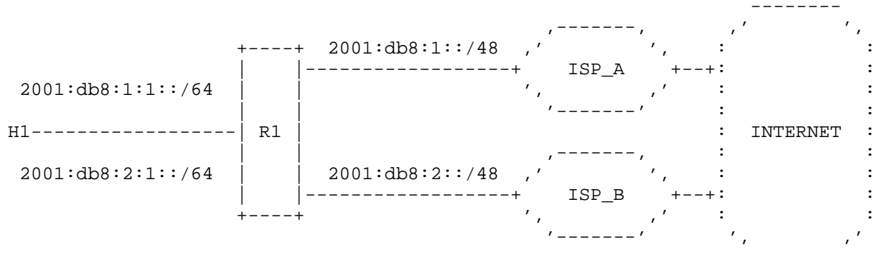
Figure 1: Single Router, Primary/Backup Uplinks
