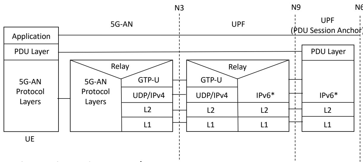
At the N3 the packet is IPv4/GTP.
