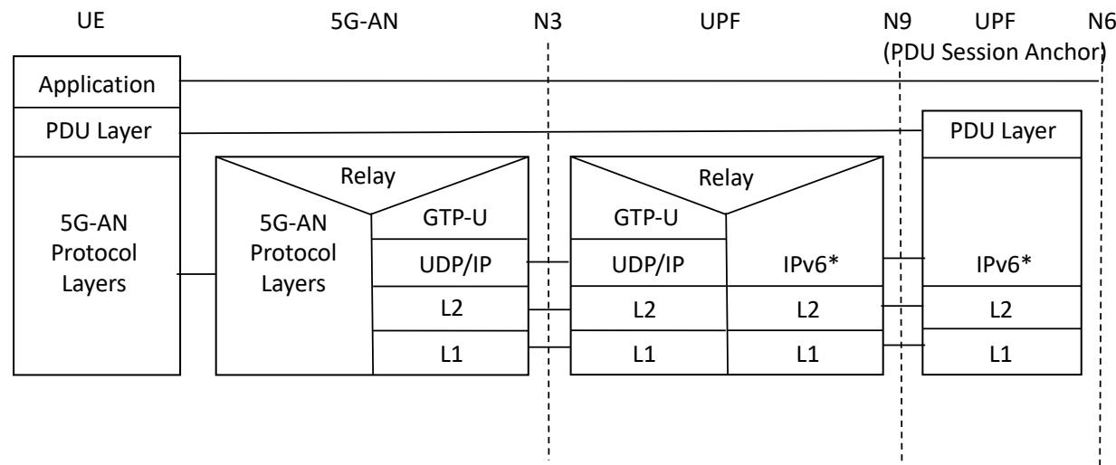
\*: IPv6 header + SRH (variable size: 1 SID = 16Bytes)
