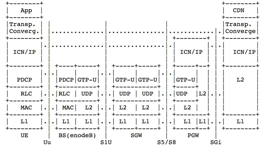
Fig. 6. Dual stack ICN Deployment in UE
