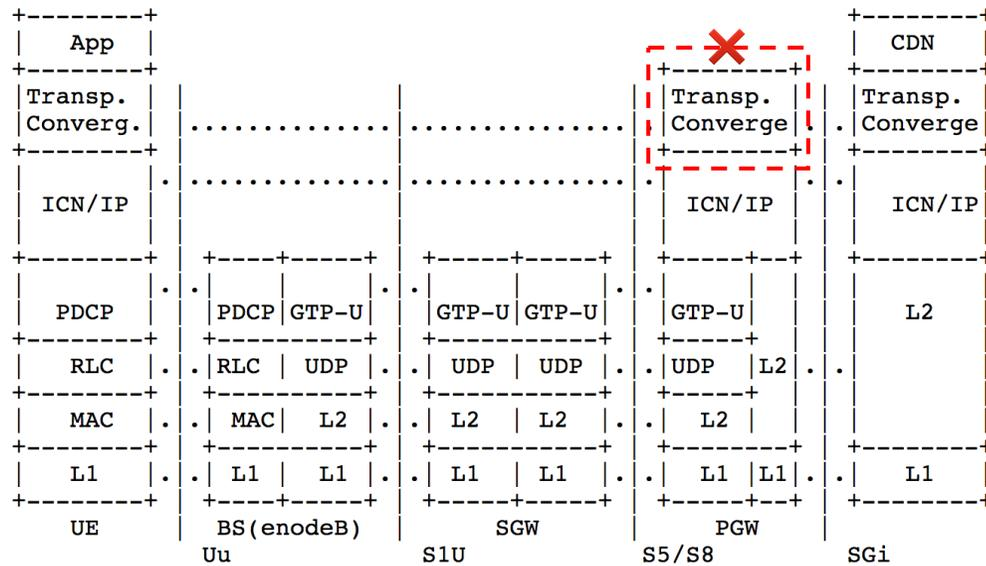
Fig. 6. Dual stack ICN Deployment in UE
