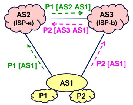
Consider data packets received on customer interfaces at AS2 with source address in P1 or P2:
