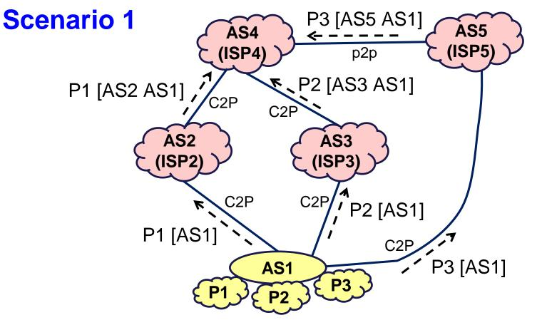
Consider that data packets (sourced from AS1) may be received on customer interfaces at AS4 with source address in P1, P2 or P3 :
