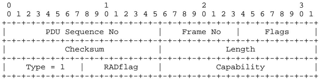
The RADflag is an integer field which signals the capability negotiation.
