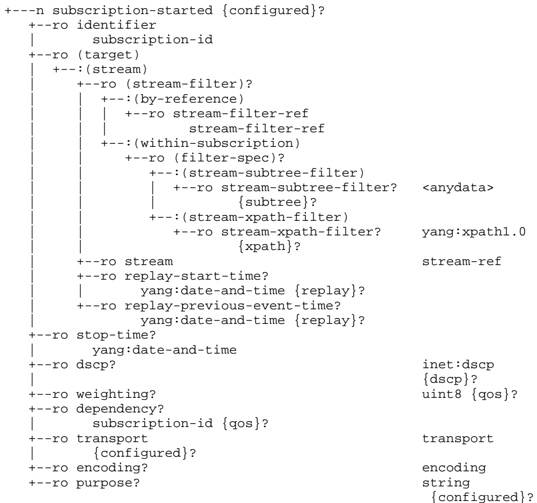
Figure 11: subscription-started notification tree diagram
