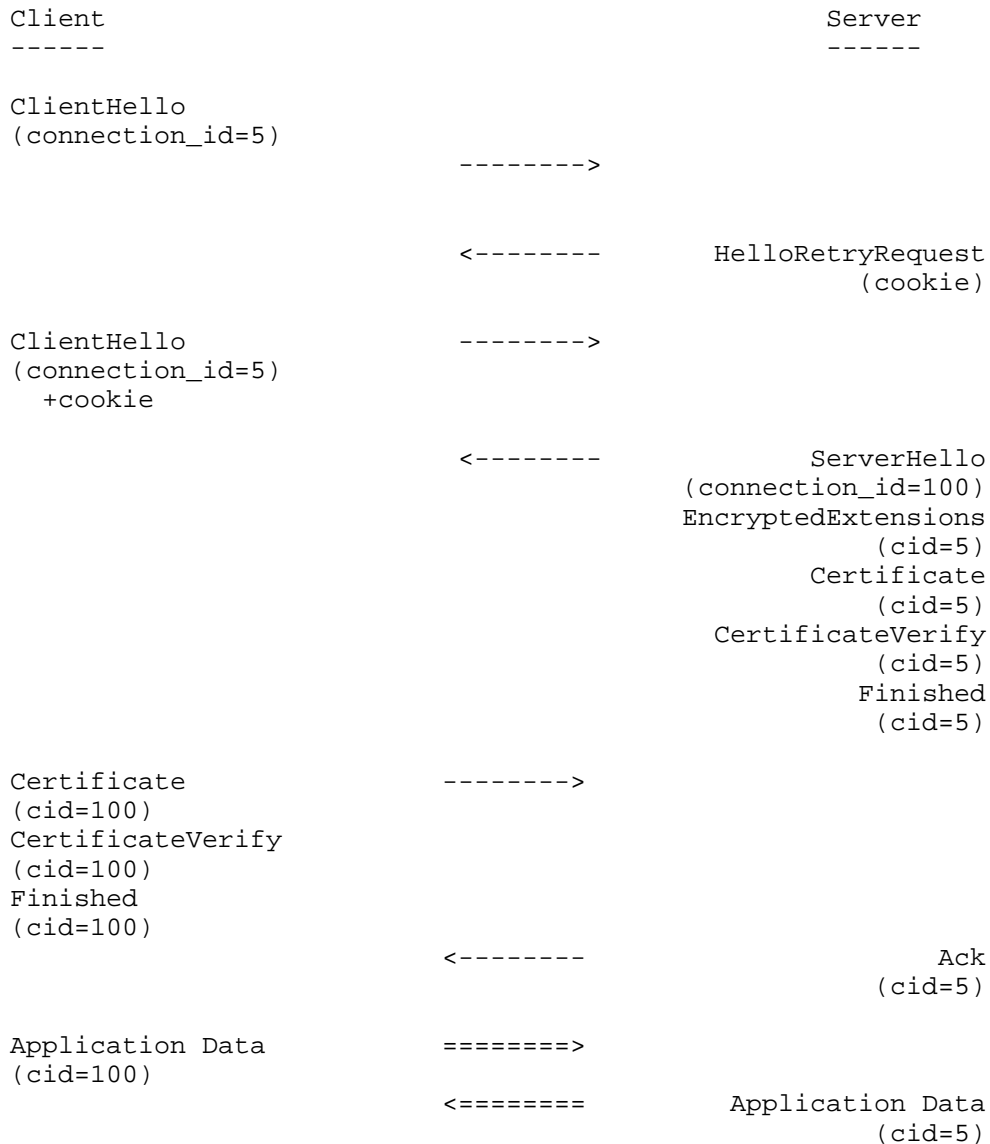
Figure 13: Example DTLS 1.3 Exchange with Connection IDs
