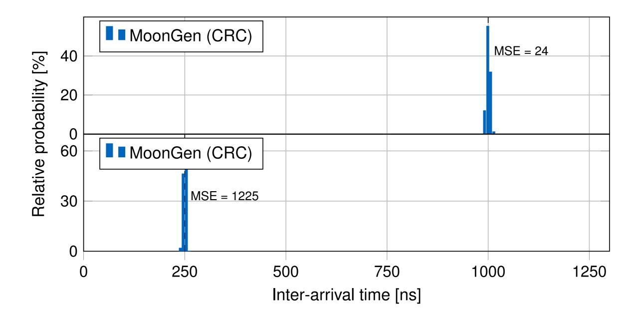
1 and 4 Mpps, MoonGen SW rate control with corrupted packets filling the gaps
