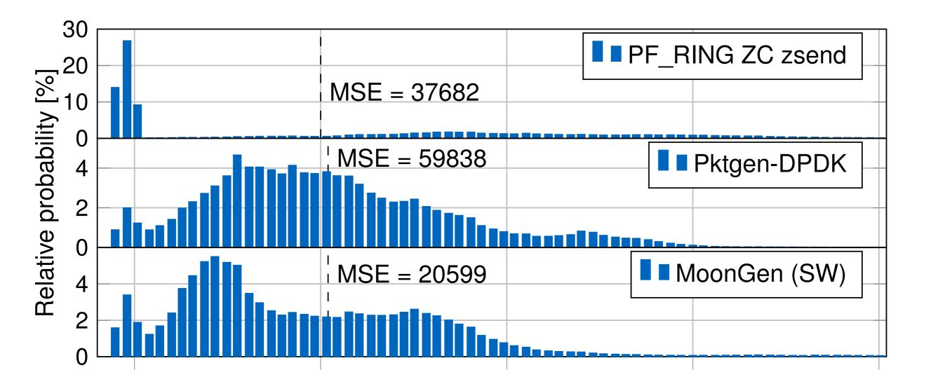
Target rate = 4 Mpps/0.25µs inter-arrival time Most packet generators fail to generate this when configured without bursts
