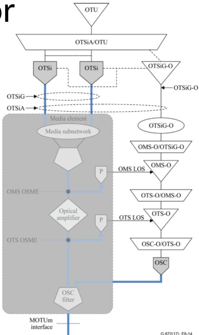
Figure 8-14 – Example of a terminal implementation using a single media element
