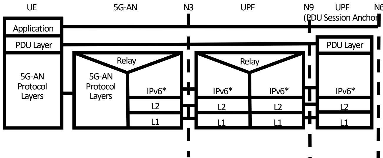
\*: IPv6 header + SRH (variable size: 1 SID = 16Bytes)
