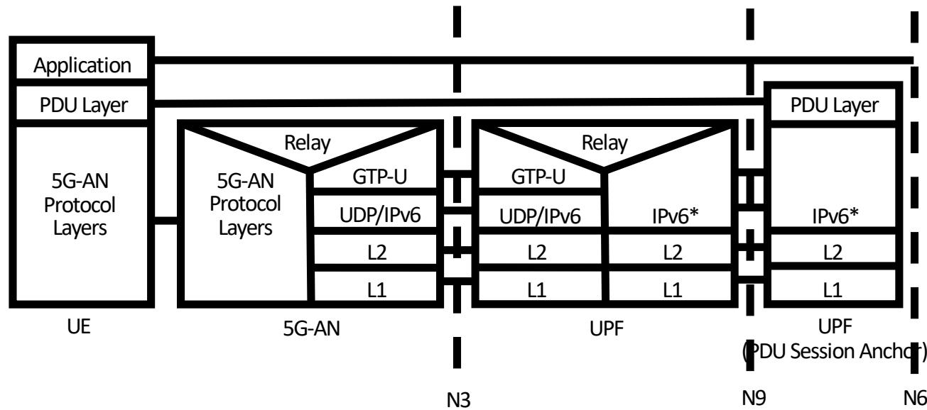
At the N3 the packet is IPv6/GTP, but IPv6 DA is an SRv6 segment. Routing is based on SRv6.
