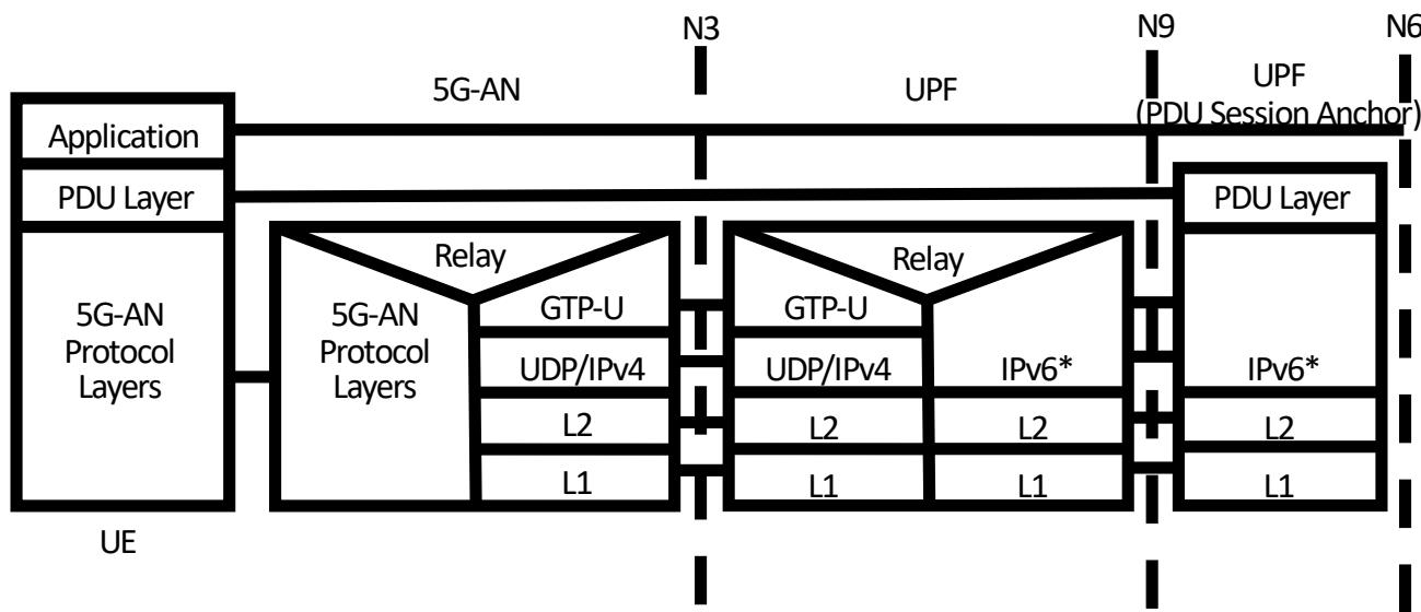
At the N3 the packet is IPv4/GTP.
