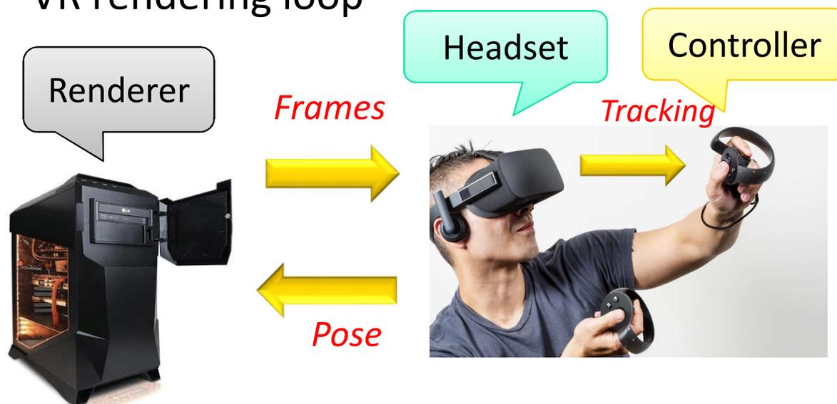
Typically, a VR system contains three key components working together (rendering loop):
