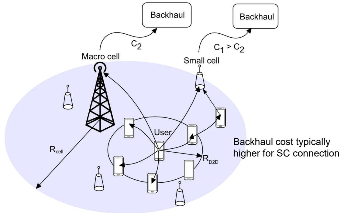
*Wireless HetNet with device-to-device (D2D) users, small cell (SC), macro cell (MC) Base Stations (BSs), and connections to backhaul*
