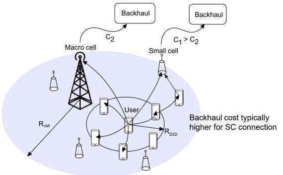
Wireless HetNet with device-to-device (D2D) users, small cell (SC), macro cell (MC) Base Stations (BSs), and connections to backhaul
