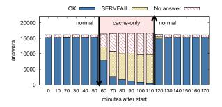
Figure: Scenario B: 100% failure after 60min, TTL: 60min
