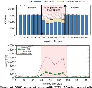
**Good**! Even at 90% packet loss with TTL 30min, most clients (60%) get an answer!! **Thanks IETFers! Good Engineering!**
