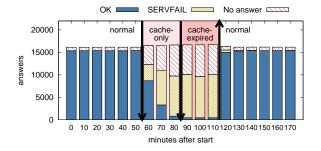
Figure: Scenario C: 100% failure after 60min, TTL: 30min
