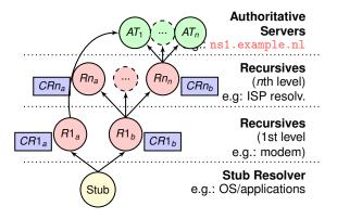
Figure: Relationship between stub resolver (yellow), recursive resolvers (red) with their caches (blue), and authoritative servers (green).
