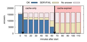
Figure: Scenario A: 100% failure after 10min, TTL: 60min
