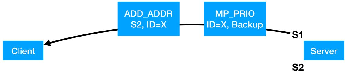
v9 removed the address-ID from MP\_PRIO (protect against attacker injecting MP\_PRIO for other paths)
