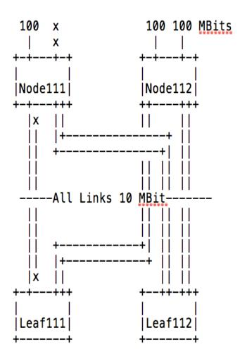
•RIFT calculates the amount of northbound bandwidth available towards a node compared to other nodes at the same level and adjusts the default route distance accordingly to allow for the lower level to have different weights on load balancing.
