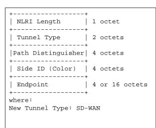
The Remote Endpoint and Color sub-TLVs, as defined in [I-D.ietf-idr-tunnel-encaps] are used to represent Site ID and CPE System ID.
