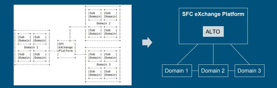
Multiple SFC domains connected by a SFC eXchange Platform
