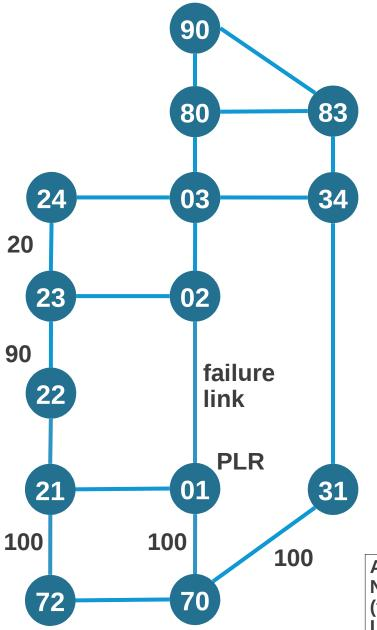
Node 70 sends packet on outgoing intf 70->01 with label stack = [701002, 102080, 180083, 183090] to instantiate path 70->01->02->03->80->83->90
