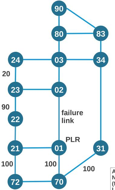
Node 70 sends packet on outgoing intf 70->01 with label stack = [101002, 102080, 180083, 183090] to instantiate path 70->01->02->03->80->83->90
