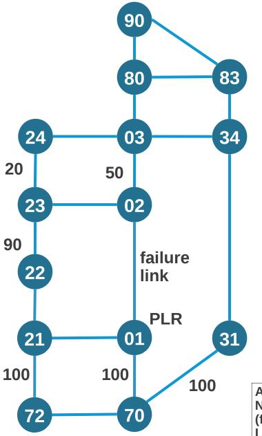
Node 70 sends packet on outgoing intf 70->01 with label stack = [101002, 702003, 103090] to instantiate path 70->01->02->03->80->90
